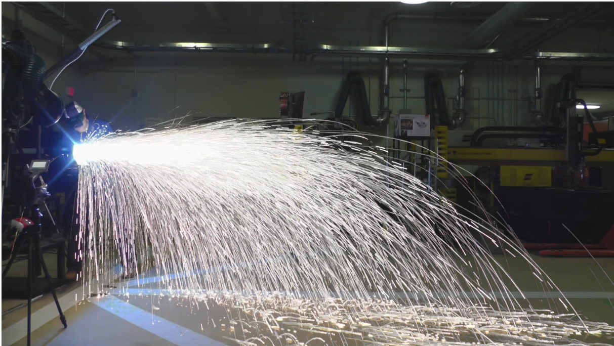
(a) Nominal plasma cutting 6mm stainless, one second composite
