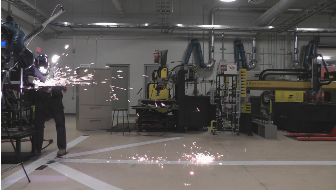
(a) Worst Case Air Carbon Arc Gouging, 25 mm carbon steel, single frame at beginning of run
