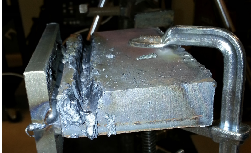
Figure 3.13: 25 mm Plate Following Horizontal Gouge
