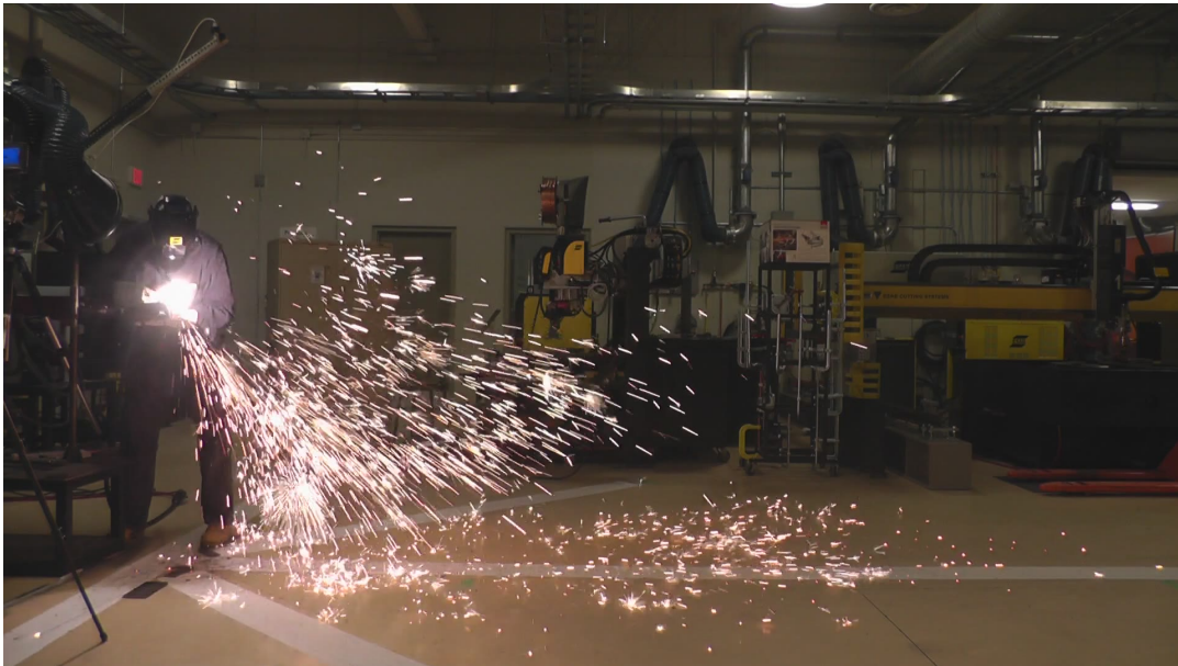
(b) Worst Case Air Carbon Arc Gouging, 25 mm carbon steel, single frame at end of run
