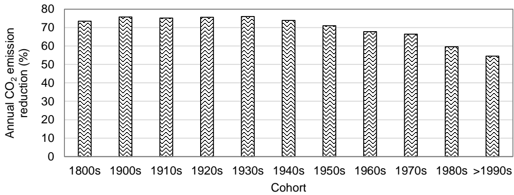
Figure 4.7: Average CO 2 emission reduction of REEP houses that have met the PH primary energy demand.
