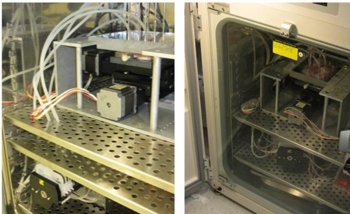
Figure 3.35 The assembled hydromechanical stimulation system shown inside incubator.
