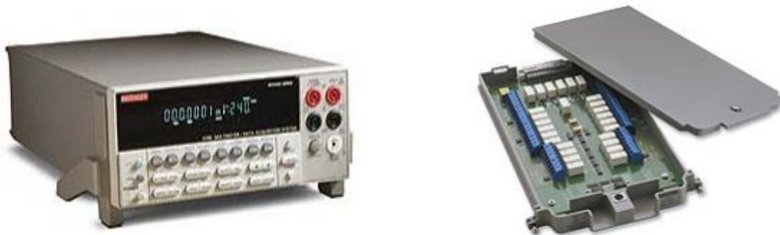
Figure 38 : Keithley 2700 data logger and M7700 input module
