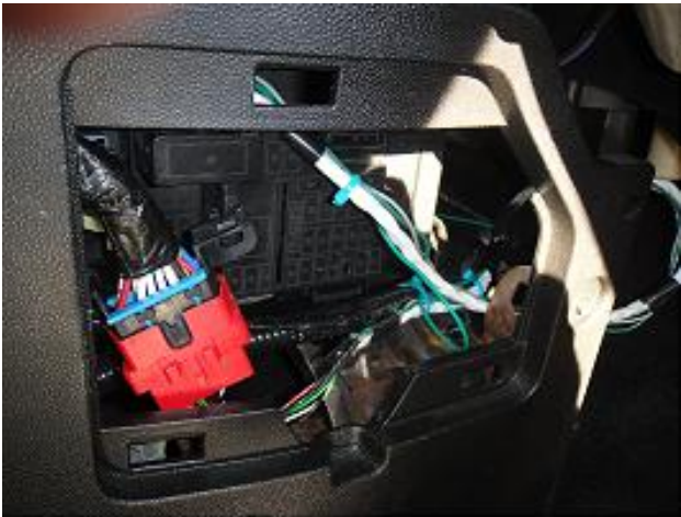
Figure 67: Data logger connection and shut down wire
