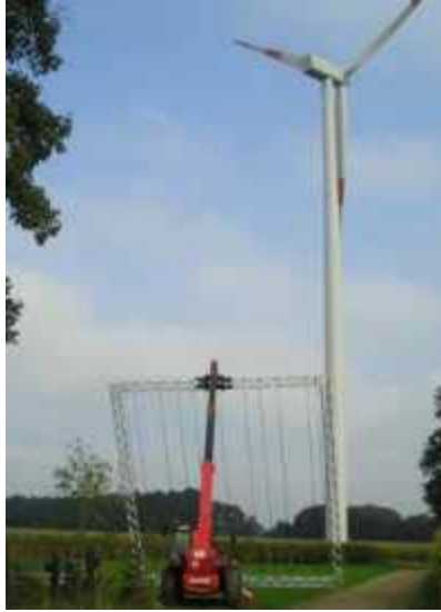
Figure 4.2: Beamforming measurement of wind turbine noise 2
