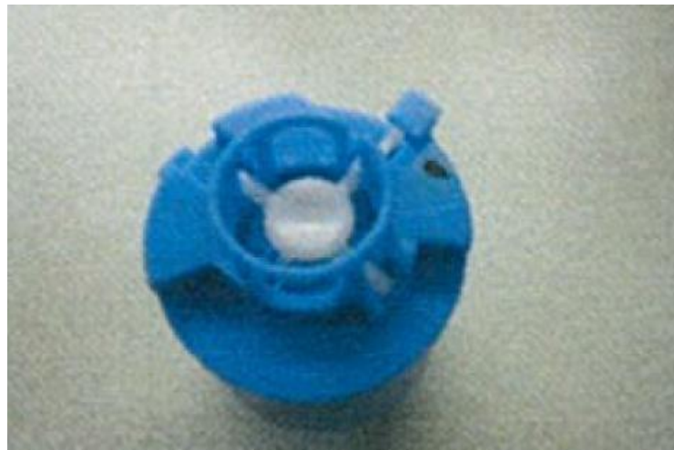
Figure 4-24: FLVV float assembly, white-satellite disc, blue-float,
