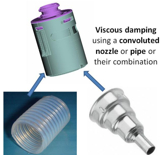
Figure 5-32: FLVV extension for damping
