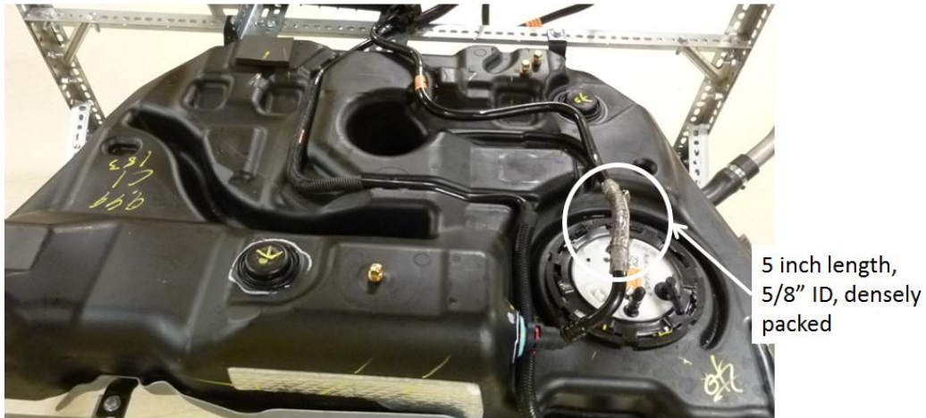
Figure 5-38: Porous material added onto tank-to-canister line
