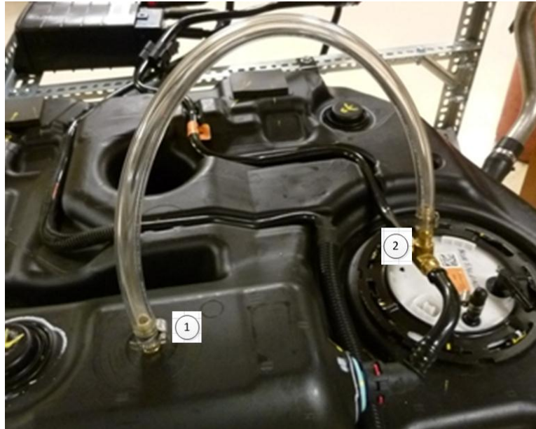
Figure 4-14: Connecting tube- tank inside and tank-to-canister line
