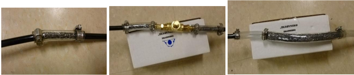
Figure 5-3: Left: 2-inch 3/8 ID tube; Middle: 4-inch 3/8 inch ID tube; Right: 5-inch 5/8 inches ID tube. All tubes are densely packed with steel wools
