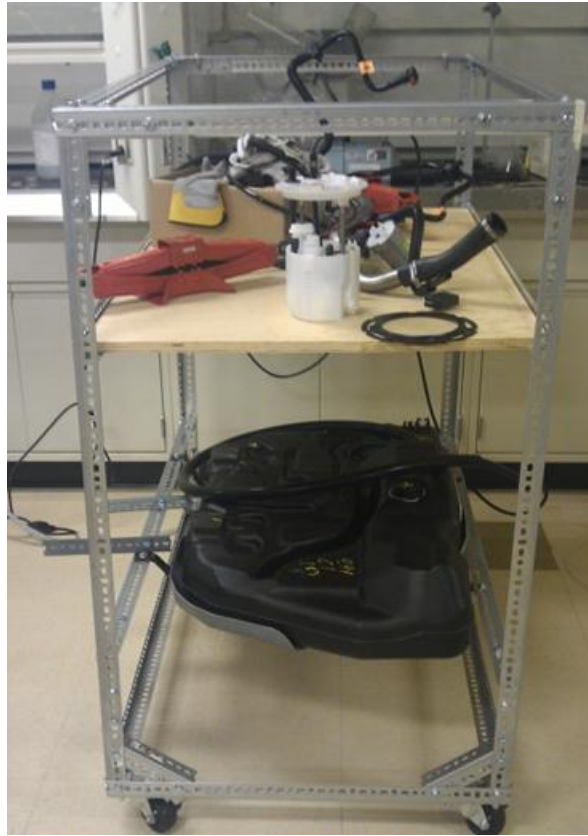
Figure 3-7: Test Rig with fuel tank mounted
