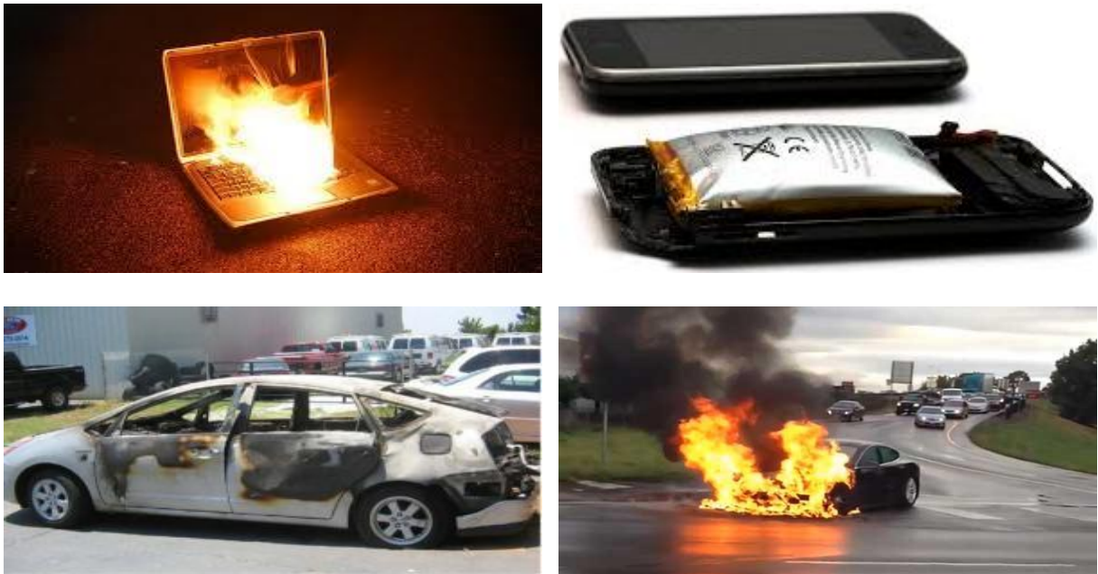
Figure 2. 5 Accidents with Li-ion batteries
