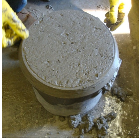
Figure 3.14: Vessel used in Air Content and Density Testing
