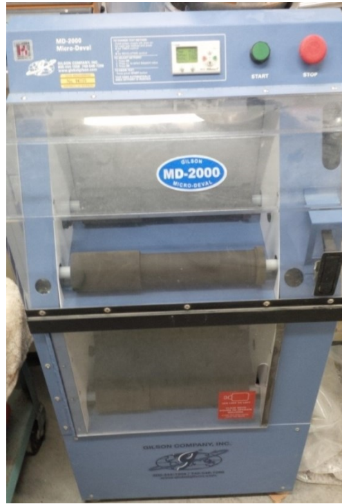
Figure 3.7: Micro-deval abrasion testing apparatus
