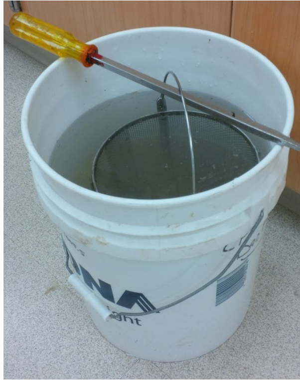
Figure 3.5: Small scale aggregate soaking
