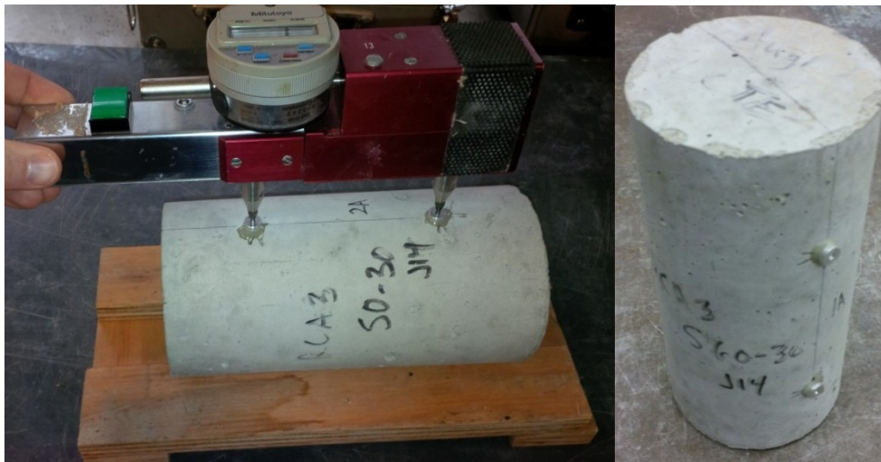
Figure 3.20: LCTE sample and testing procedure
