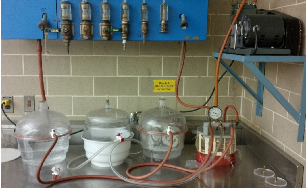
Figure 3.21: Permeable porosity testing assembly
