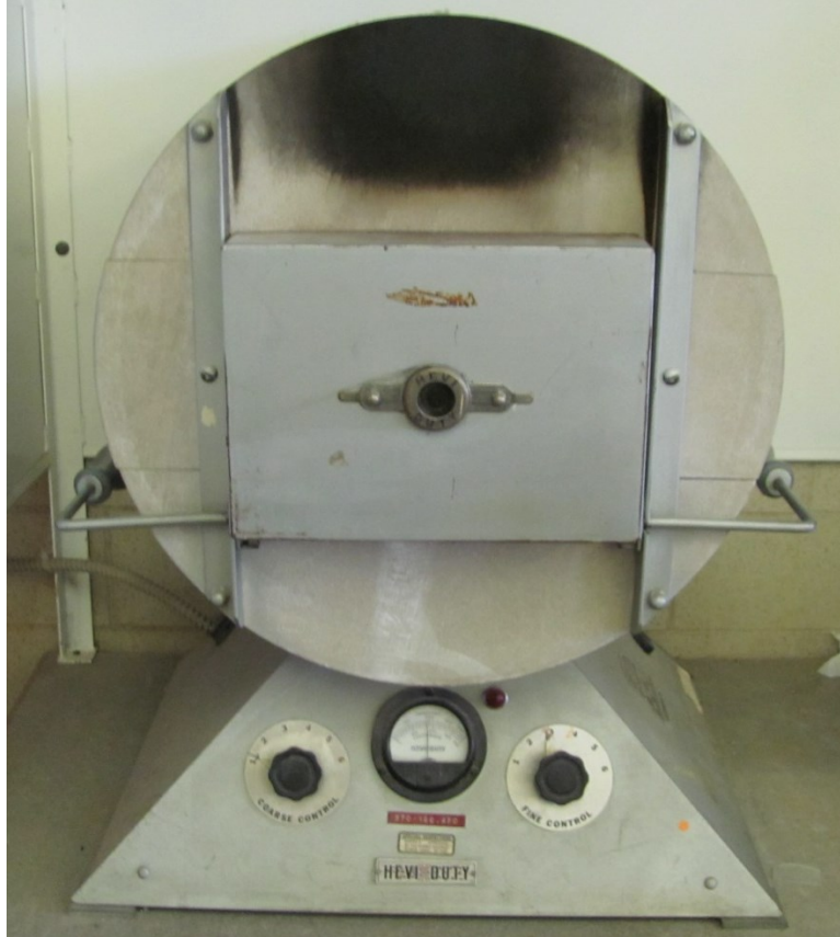
Figure 3.3: Muffle furnace employed in the adhered mortar test procedure
