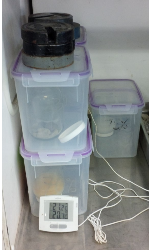
Figure 3.6: Air-tight, controlled RH environments
