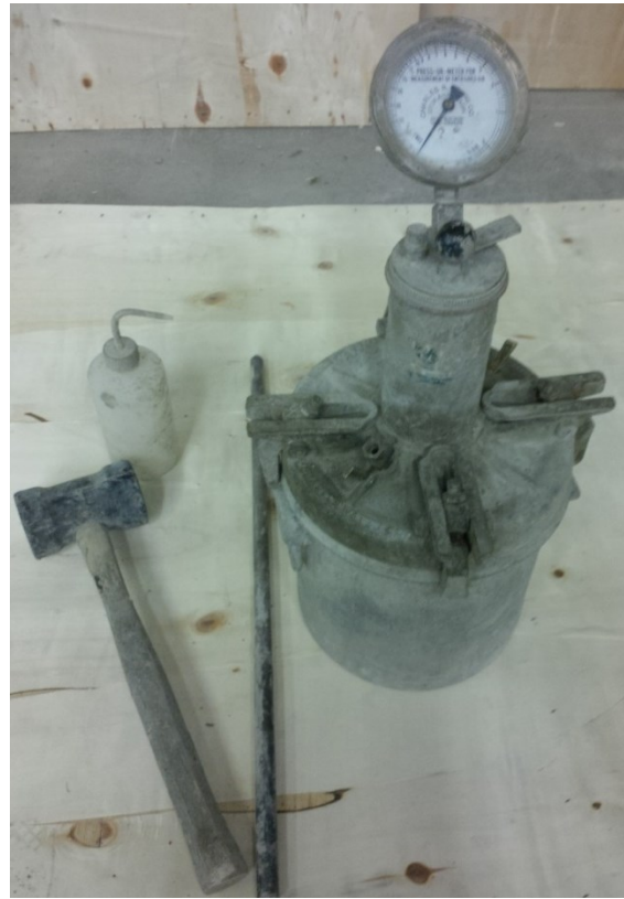
Figure 3.13: Air meter and associated equipment for air content testing
