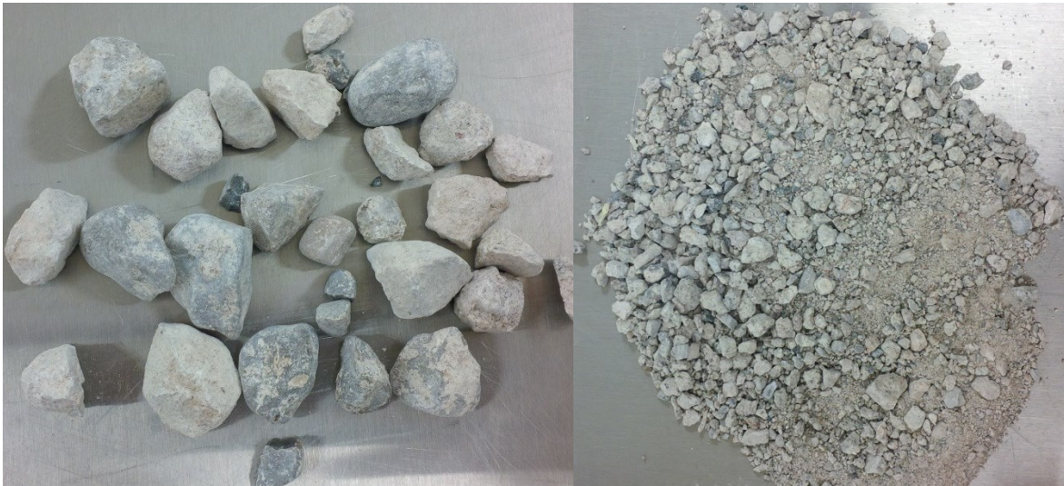
Figure 4.2: Sample of RCA2 after removal of adhered mortar
