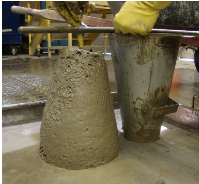
Figure 3.12: Slump measurement of fresh concrete
