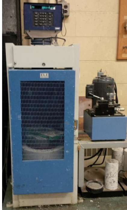
Figure 3.15: Compressive strength testing machine
