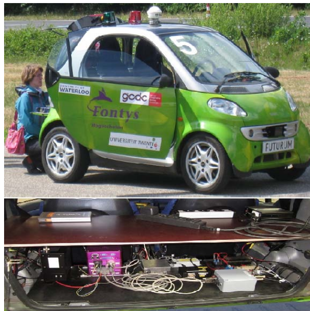
Figure 5.1: Test vehicle for testing platooning strategies
