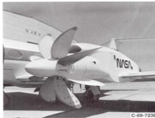
Figure 4: SR-7L propeller on the Gulfstream II aircraft [47]
