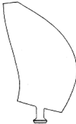
Figure 41: Shape of the SR-7A propeller blade [42]
