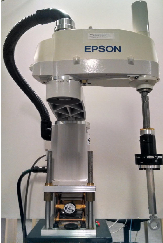
(a) Photograph of Epson SCARA Robot used for Radial Flux Measurement.
