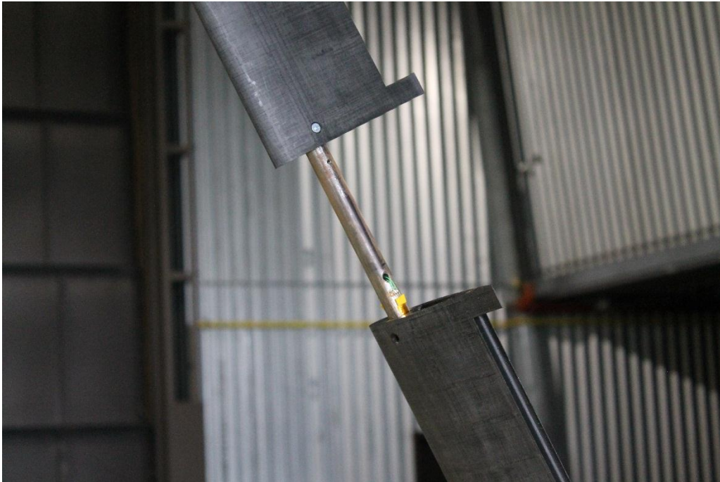
Figure 5.7. Image showing flap section sliding into position.
