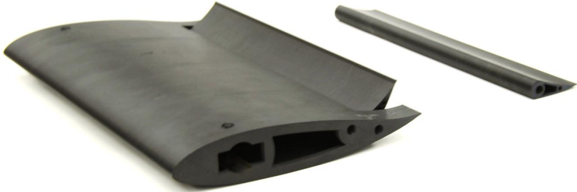
Figure 4.10 Image of printed blade flap section and trailing edge flaps.
