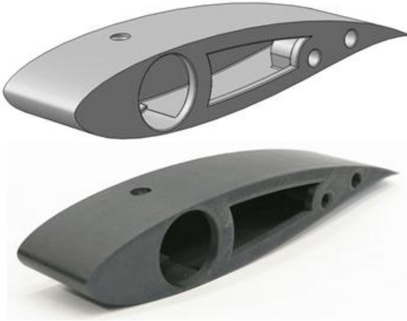
Figure 4.2 3D model vs. photo of manufactured prototype of the blade tip section.
