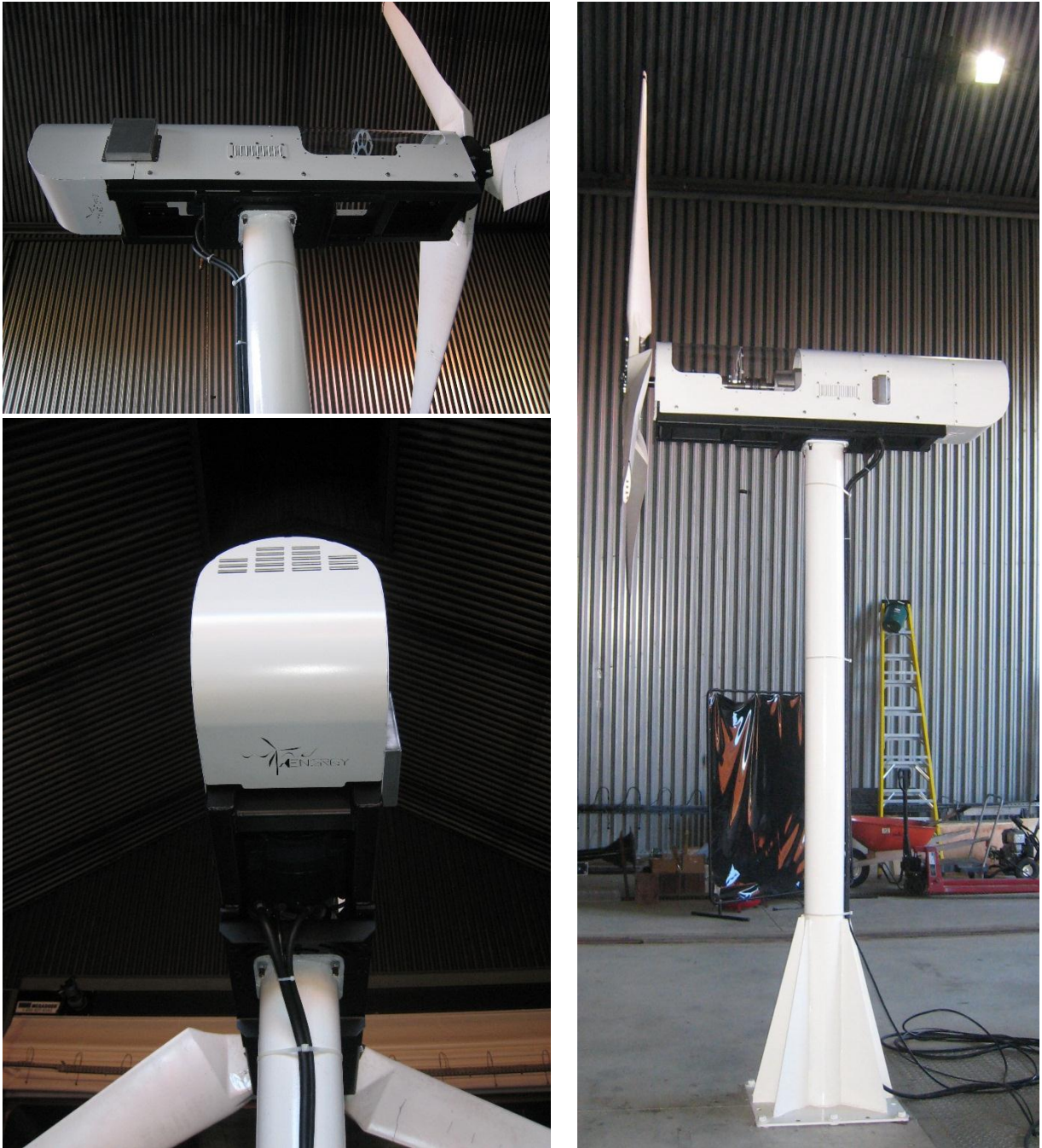
Figure 3.19 Fully assembled wind turbine test rig images with Gertz [34] rotor.
