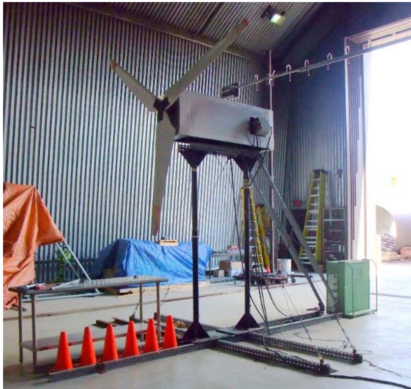
Figure 3.1 Image of previous Test Turbine Rig
