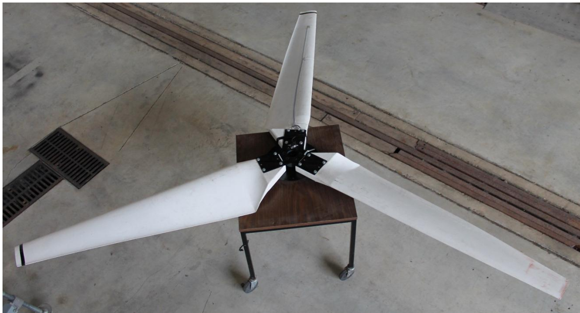
Figure 3.10 Image of assembled rotor using new hub design and Gertz [34] blades.
