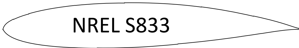
Figure 4.1 NREL S833 airfoil [51].
