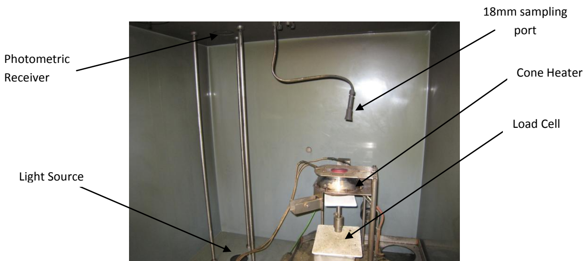
Figure 3.6: Detail of the interior of the UWLFR Smoke Density Chamber
