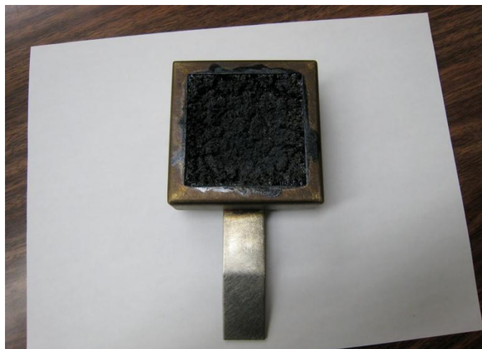
Figure 4.32: Char residue of 20%EGFR sample after smouldering in the smoke density chamber
