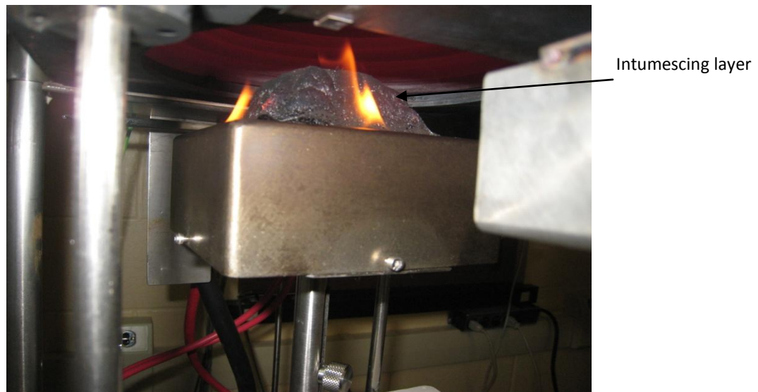
Figure 4 .4: 10% EGFR under the action of 50\text{kW/m}^2 heat flux in cone calorimeter testing
