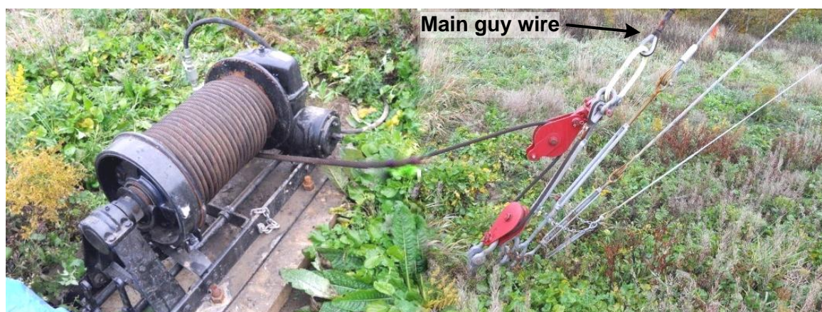
Figure 1.4: The winch at left, operated by a hydraulic pump (not shown), enables the lowering and raising of the wind turbine using the main guy wire after the others are removed.
