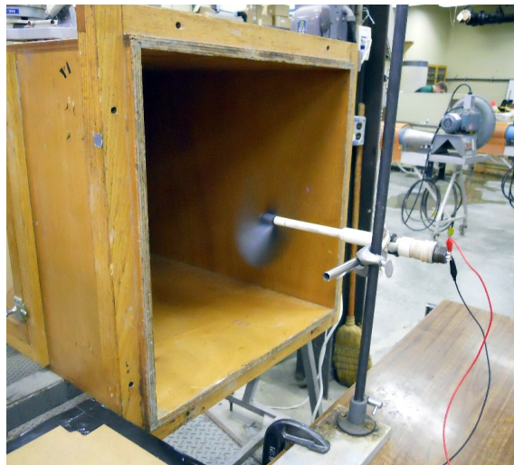
Figure A.4: Propeller anemometer test setup in open jet wind tunnel with black carbon fibre propeller.
