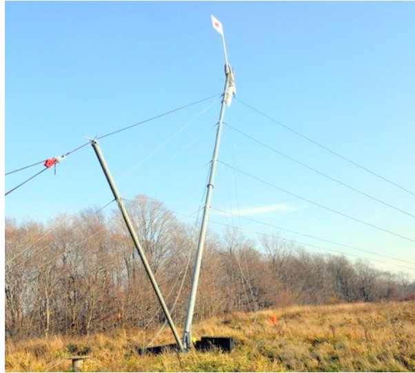
Figure 1.5: The tilt-down function of the Wenvor wind turbine makes for comparatively simple maintenance and installation of instrumentation.
