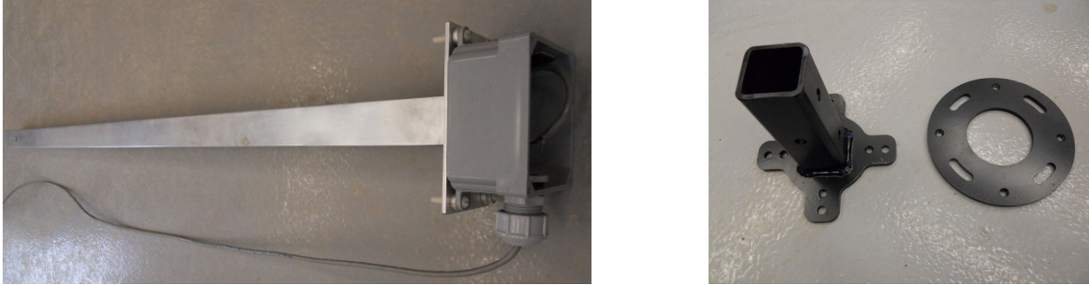
Figure A.8: The digital compass is in the box fixed to a 1.1 m aluminum pole to remove it from magnetic induction fields produced by the generator. It is attached to the top of the tail with the mounts shown at right, which allow for small adjustments of the orientation in the field to account, for instance, for magnetic declination of approximately 10^\circ at the site.
