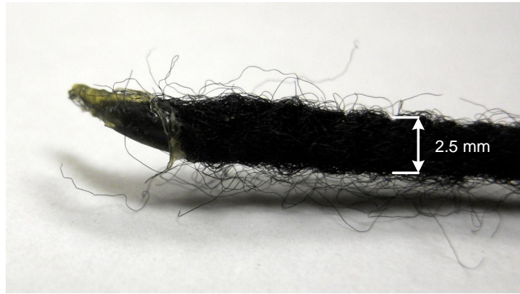
Figure 3.10: Close-up of hot glue on a tuft used to keep the tip from fraying.
