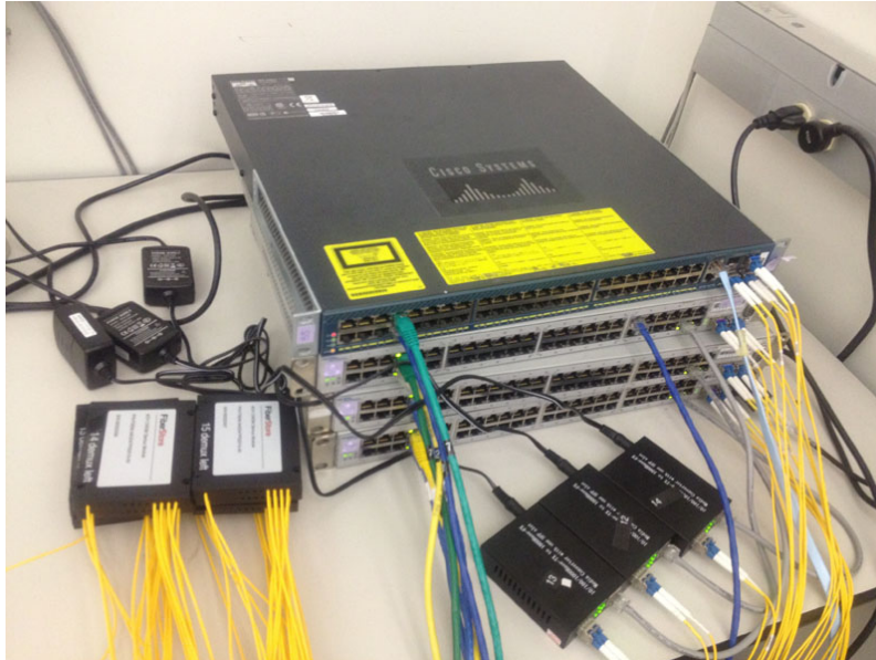
Figure 4.4: Quartz with 4 switches, connected by WDMs
