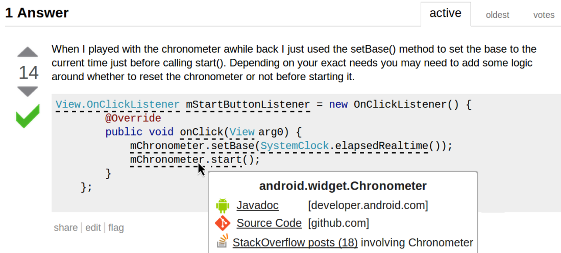
Figure 4.6: Baker-augmented Stack Overflow post. Note that the Baker browser extension automatically augmented the Stack Overflow post without any intervention from the teams maintaining Stack Overflow, Github, or the Android documentation.
