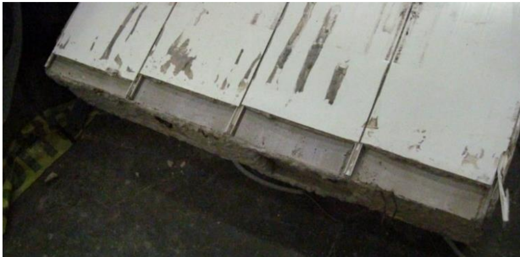
Figure 4.16: Tested specimen showing tension panel slip (PH-6-10)
