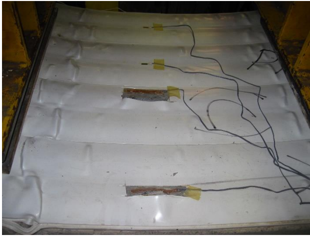
a – Failure by steel yielding followed by concrete crushing then PVC bubbling then rupture of PVC panel. (PF-7-10)
