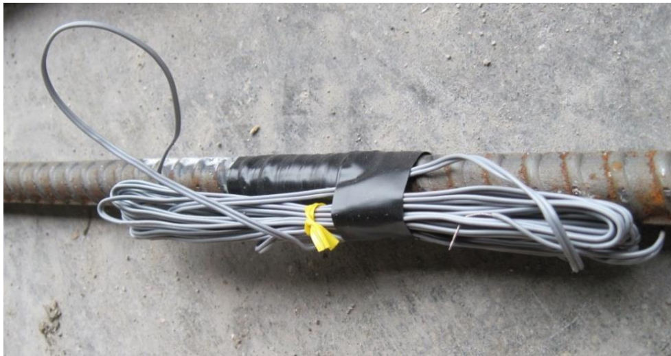
Figure 3.11: Protected strain gauge before assembly
