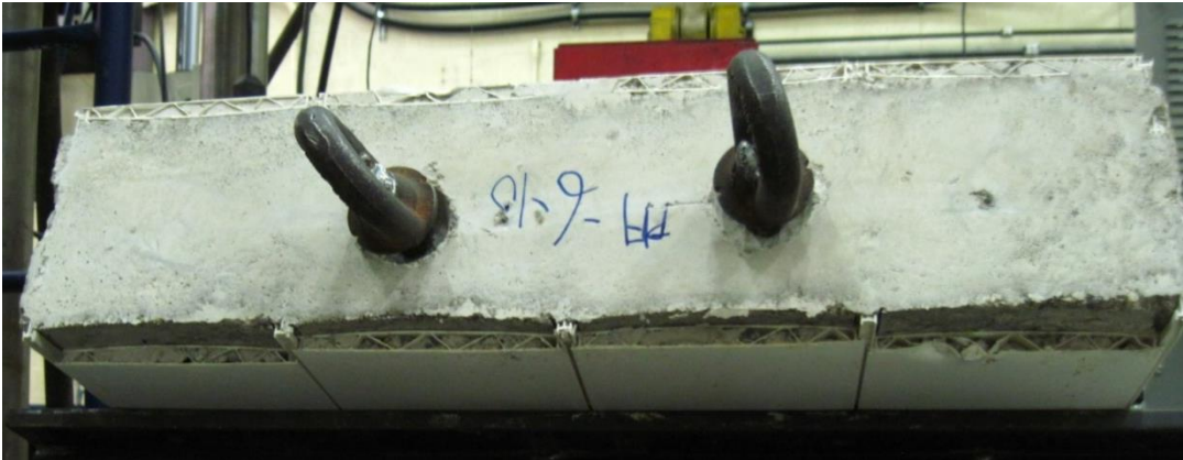
Figure 4.26: Panel slips observed on wall PH-6-10
