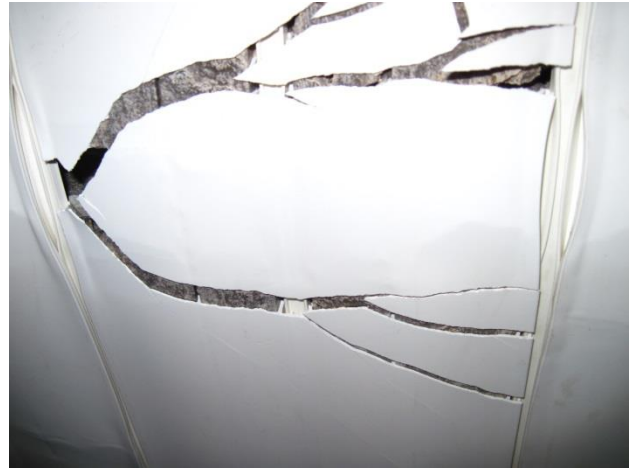
a – Failure by steel yielding followed by concrete crushing then PVC bubbling then rupture of PVC panel. (PF-7-10)
