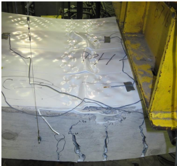
Figure 4.15: Bubbling on PVC surface and buckling of compression panel (PH-8-10)
