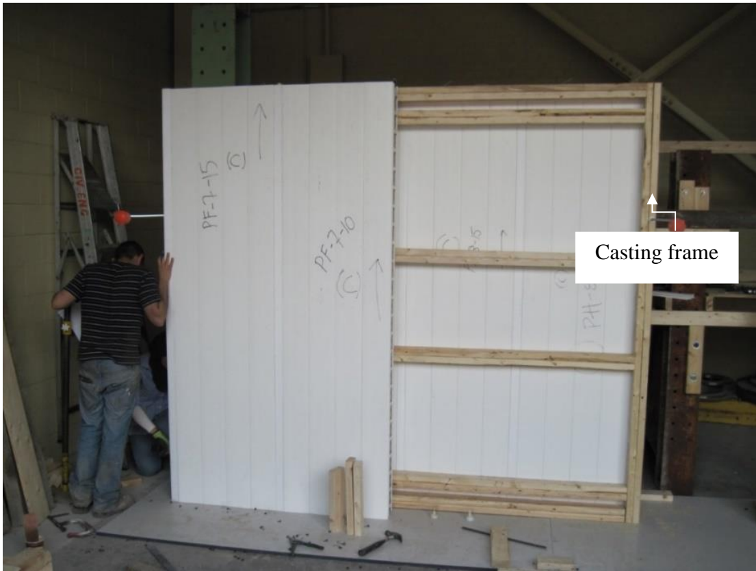
Figure 3.4: Wall specimens tilted into place
