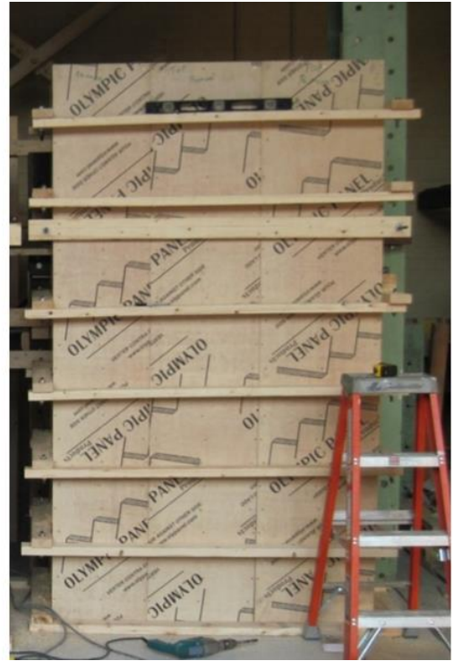
Figure 3.3: Placing the reinforcing steel inside control box; final assembly of the three control boxes with timber girdling
