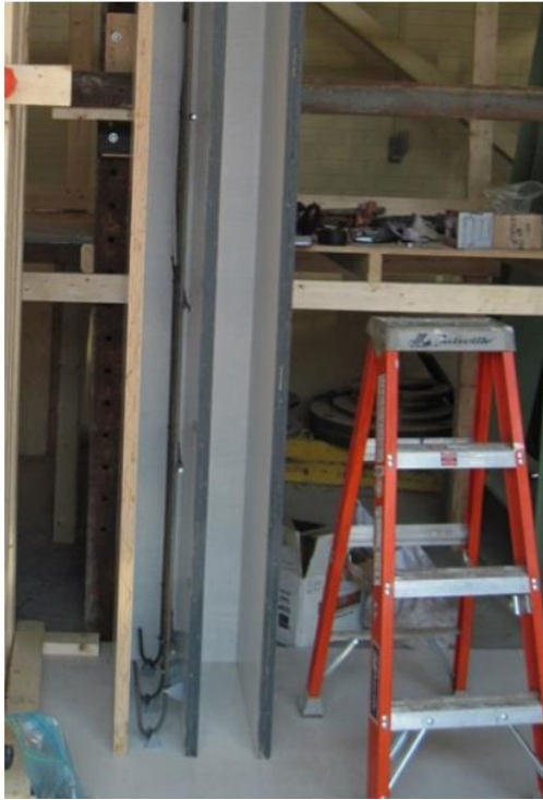
Figure 3.3: Placing the reinforcing steel inside control box; final assembly of the three control boxes with timber girdling
