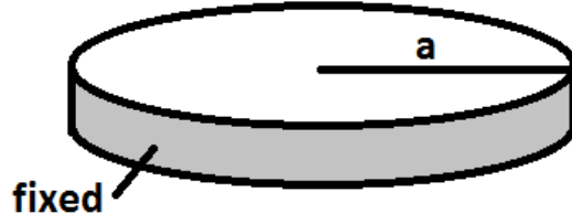
Figure 3.1: The basic shape of a circular CMUT membrane.
