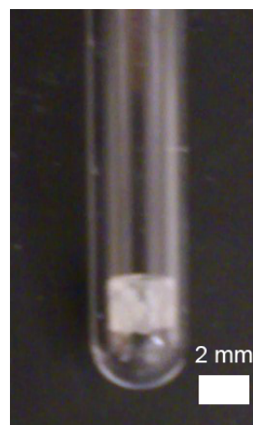
(b) Stycast box for crystal orienting.
