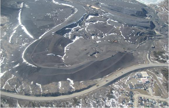
**Fig.3.35 Regrading**Earth movers regrading the slag heaps to receive liming and seeding and achieve better adherence.
