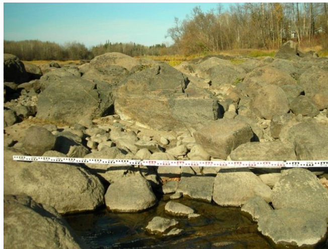
Figure C.2: Example of a Stadia Rod Photograph
