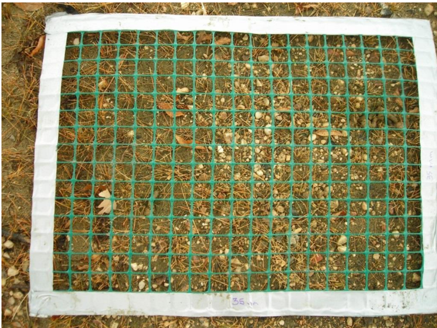
Figure C.3: Example Grid Photograph – Fines/Sand (FS)
