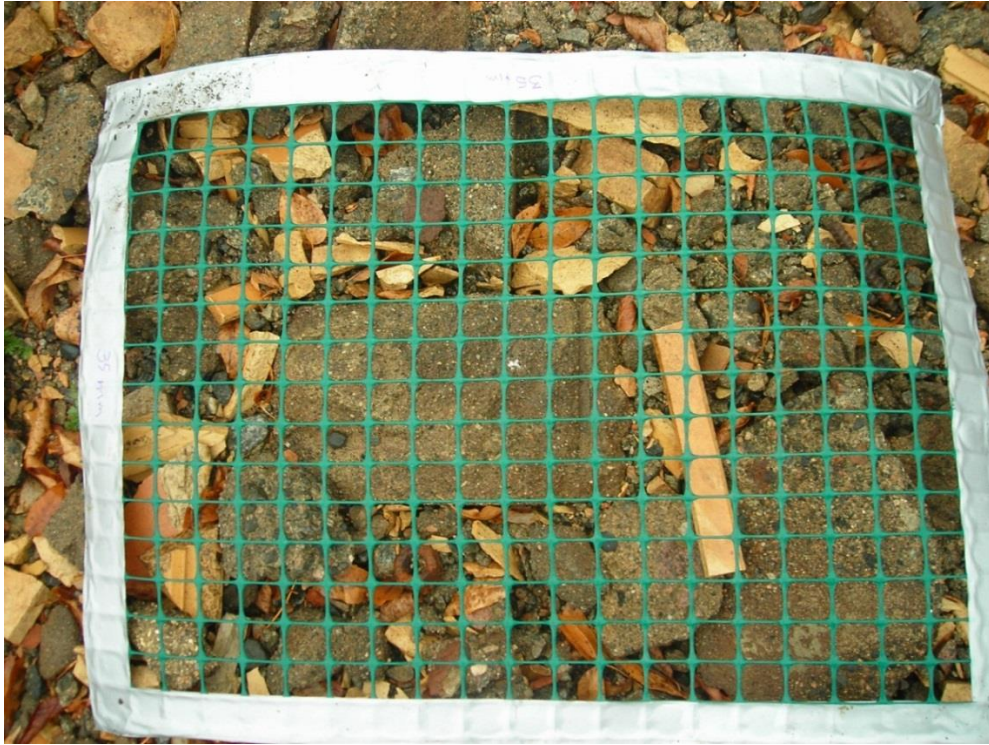
Figure C.7: Example Grid Photograph – Predominantly Gravel, with Cobbles/Boulders (G-CB)
