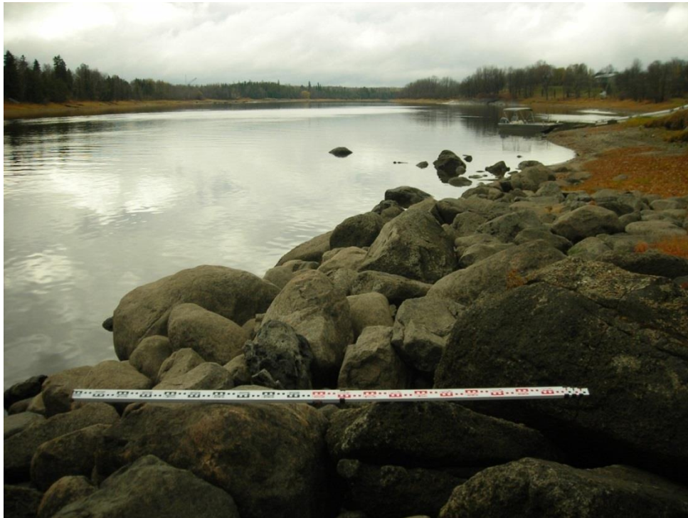
Figure C.7: Example Grid Photograph – Predominantly Gravel, with Cobbles/Boulders (G-CB)
