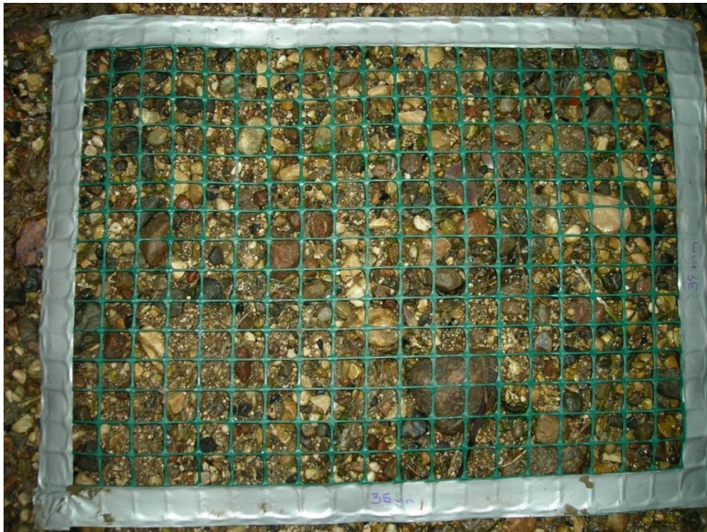
Figure C.5: Example Stadia Rod Photograph – Predominantly Fines/Sand, with Cobbles/Boulders (FS-CB)
