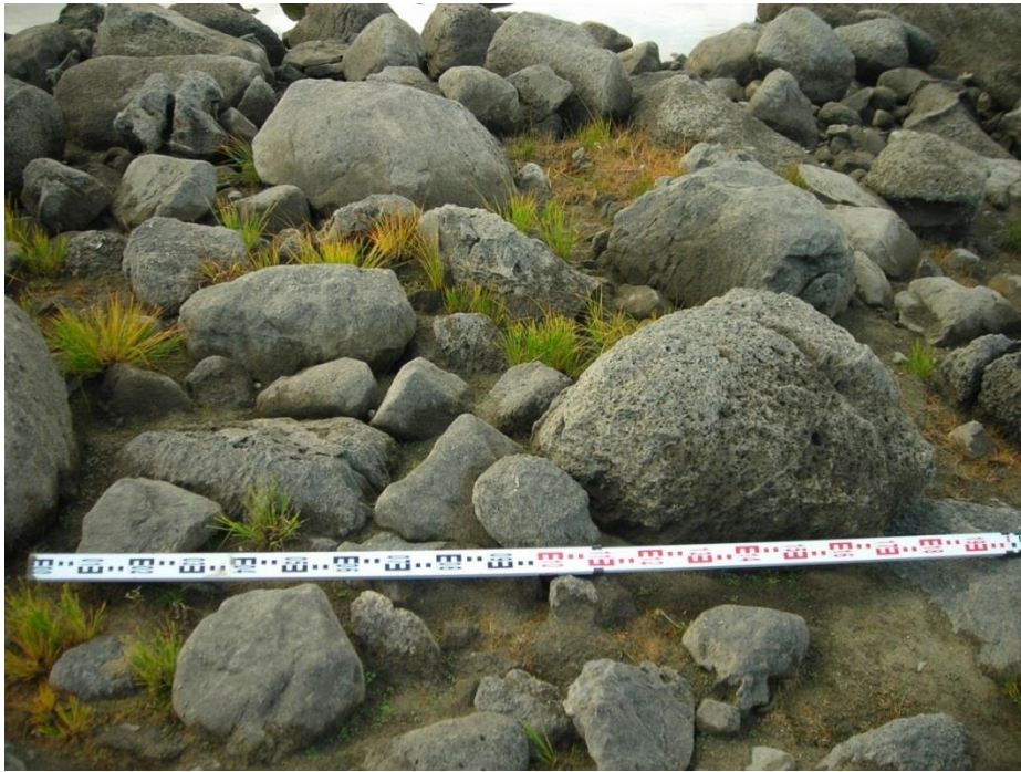
Figure C.5: Example Stadia Rod Photograph – Predominantly Fines/Sand, with Cobbles/Boulders (FS-CB)
