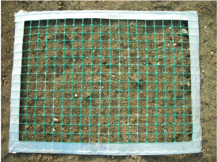
Figure C.3: Example Grid Photograph – Fines/Sand (FS)
