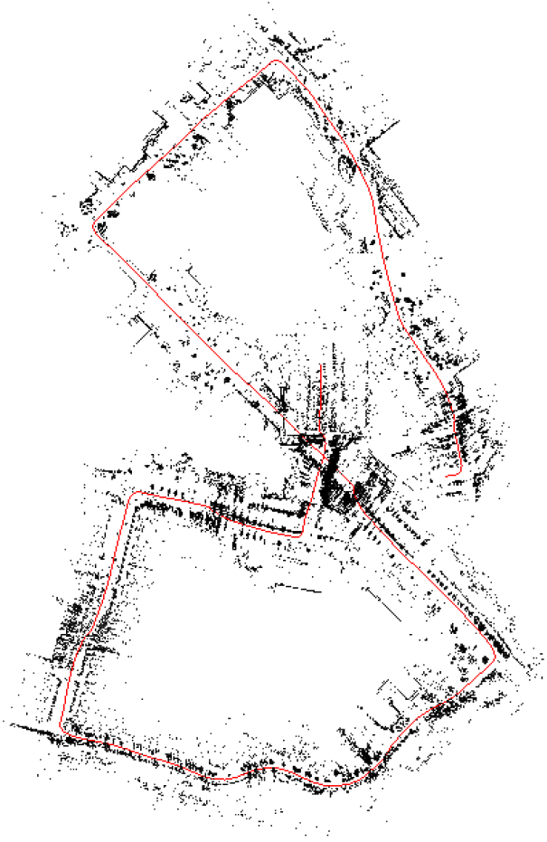
Figure 3.6: Full map generated from the Ford dataset using only scan-to-scan matching with the GSICP method. This map shows obvious drift but the local structure is very accurate.
