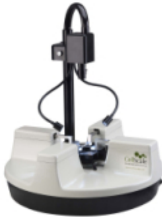
Figure 5-1 - The BioTester 5000 was used to perform biaxial testing of both single and bi-layer samples of porcine annulus tissue.
