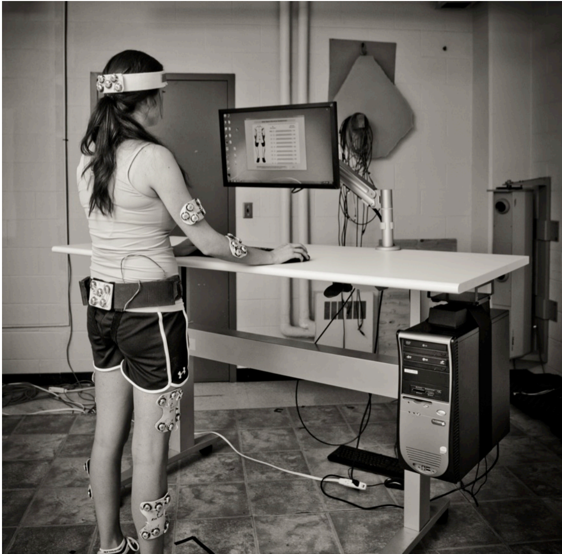
Figure 4-5 - Mockup of participant standing while completing a discomfort questionnaire. Note: Although an active marker motion capture system was used, for this mockup, markers are not daisy chained together for power as they would be for a real data collection.
