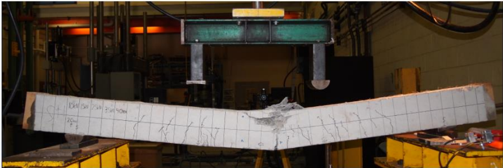
Figure 4-3 – Deformed shape of PP1 beam at failure [34]
