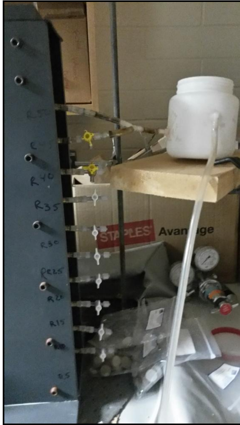
Figure 2.3 The outflow end of the sand tank showing the positions of each outflow port and the reservoir used to control the hydraulic head.
