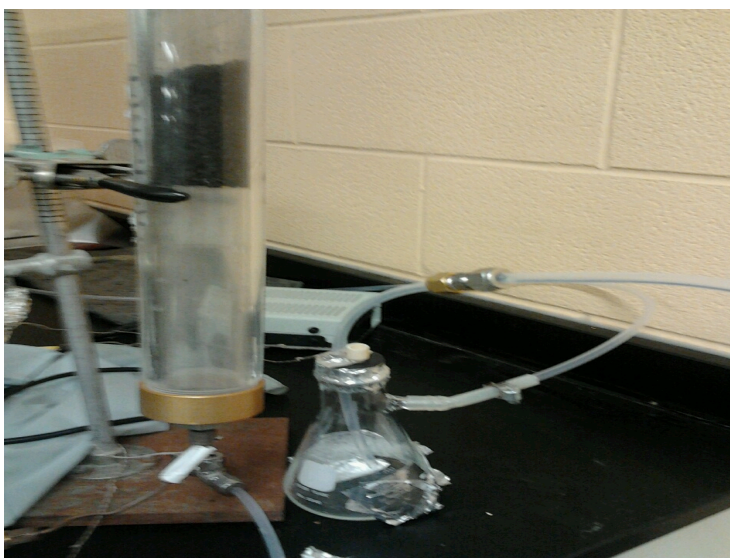
Figure 2-30: The laboratory column of activated carbon for testing continuous experiments
