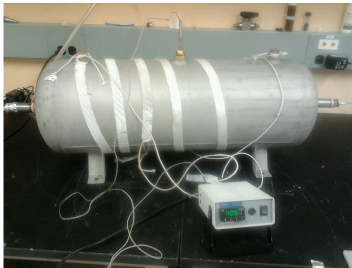
Figure 2-34: Absorber tank with electrical heating tape wrapped around for heating purpose
