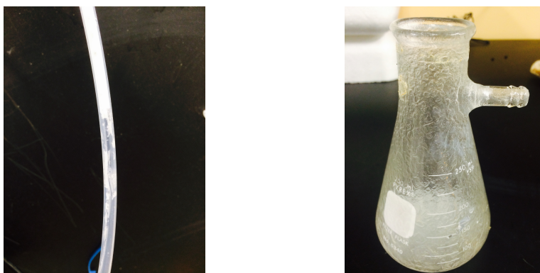
Figure 2-40: Photograph of white solid material collected in the outlet tube (left) and condenser flask (right) after several days of thermal desorption
