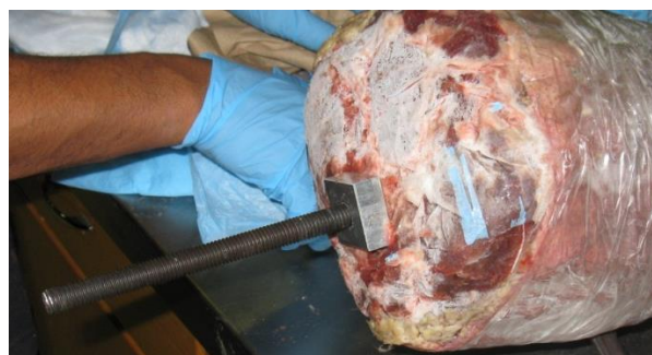
Figure 32 Locator blocks mounted on distal ends of un dissected cadaver knee
