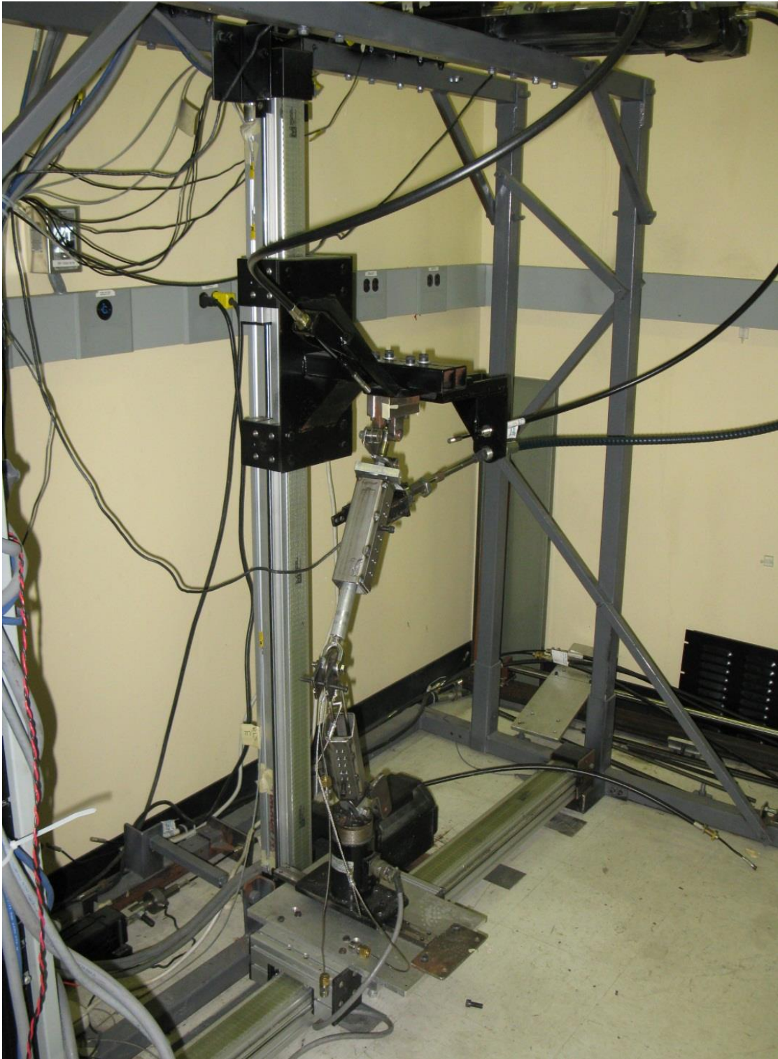
Figure 21 Mechanical knee model mounted on Dynamic Knee simulator
