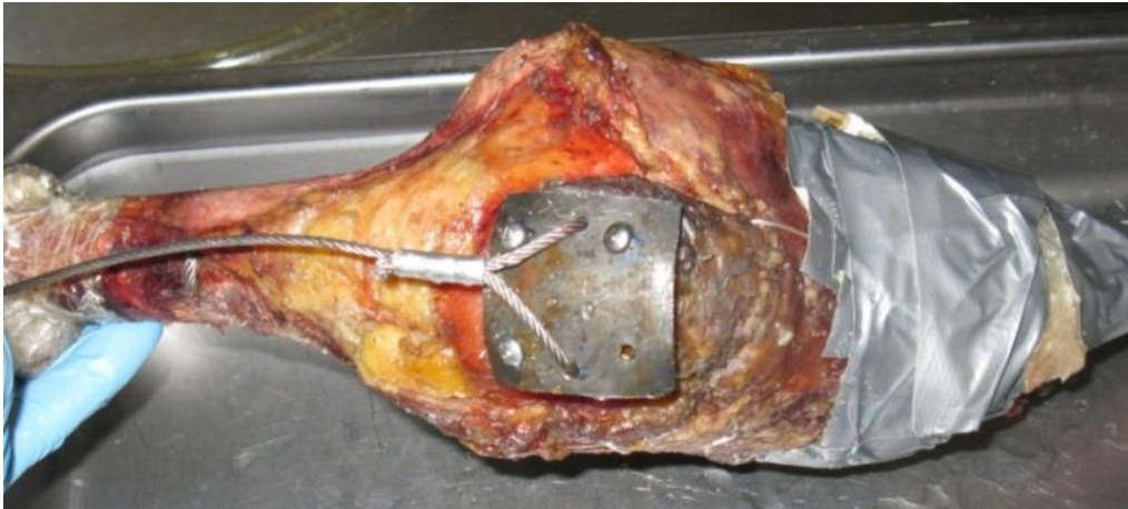
Figure 54 Quadriceps muscle actuator cable attached to patella with reinforced metal shims to avoid stress concentration (new technique of attaching quadriceps cable to patella)
