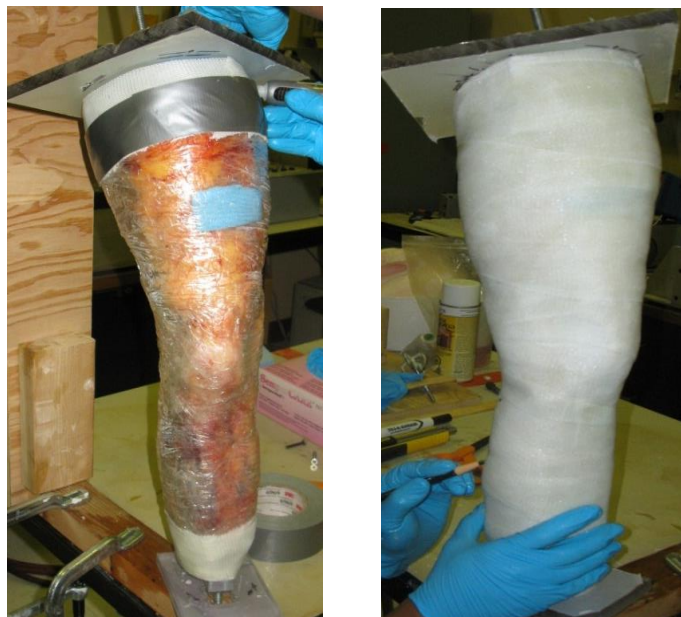
Figure 35 Creation of negative mould (“tape mould”) in shape of cadaver knee for future foam casting
