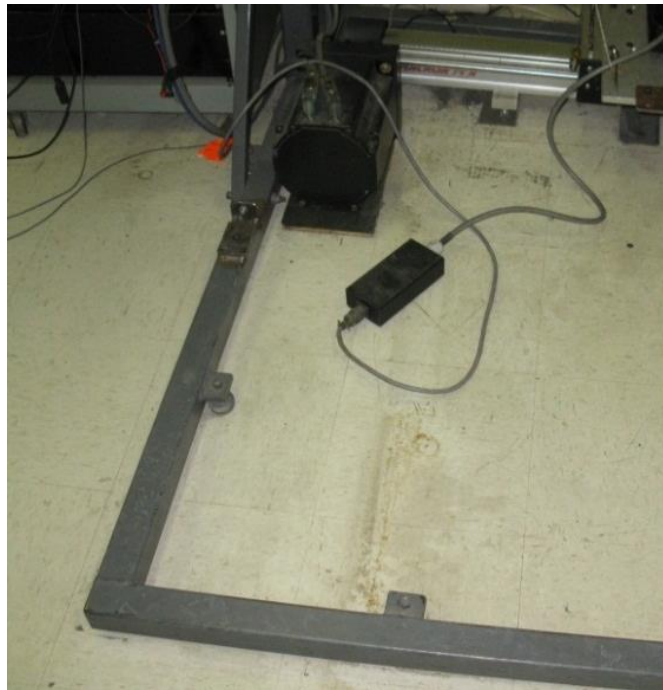
Figure 19 Leveling feet added to the actuator frame to stabilize the equipment
