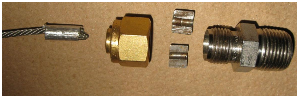
Figure 40 Cable clamp hardware in proper configuration prior to assembly
