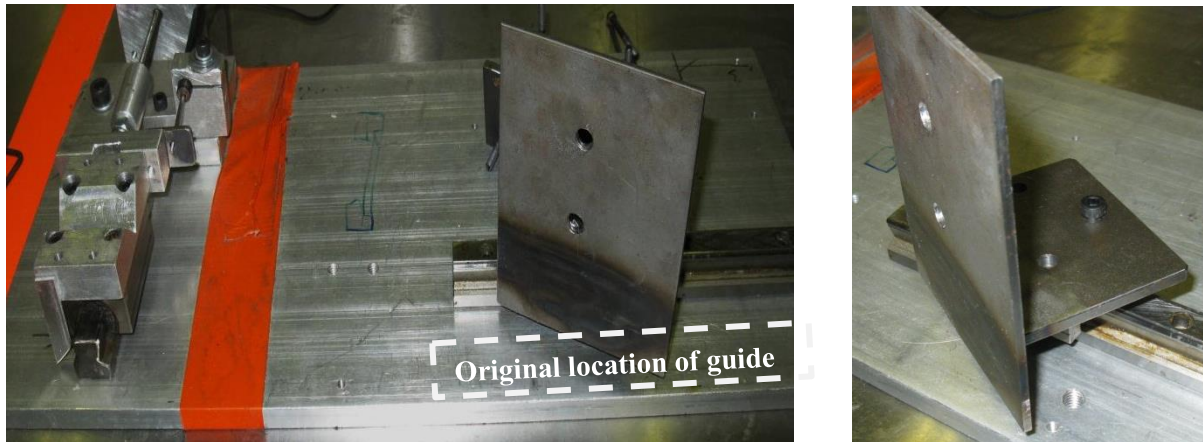
Figure 14 Modifications completed on Lachman Tester
