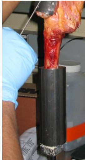
Figure 42 Metal tube encased on femur of cadaver knee for reinforcement
