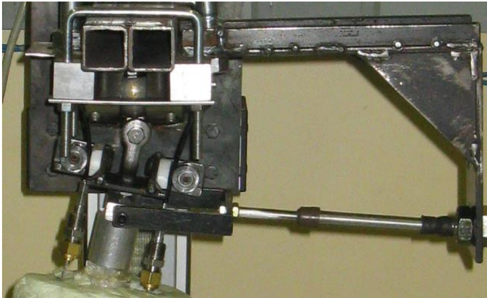
Figure 25 Muscle cable guide attachment configuration at hip joint site on Dynamic Knee simulator
