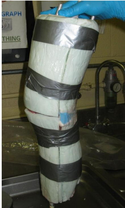
Figure 47 Hybrid surrogate specimen with foam casing encapsulating cadaver knee specimen
