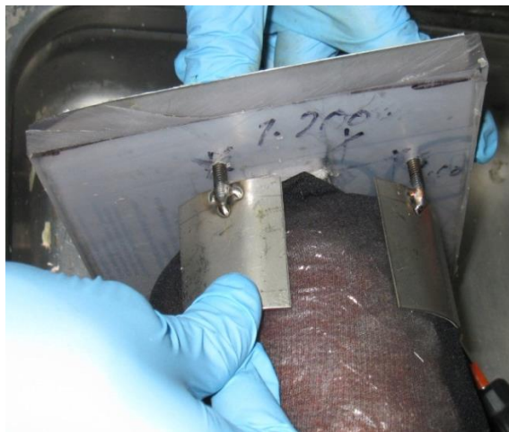
Figure 34 Locator posts inserted into end plates during preparation of tape mould
