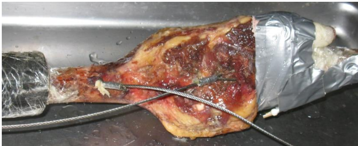
Figure 38 Cadaver knee specimen prepared with muscle force cable attachments
