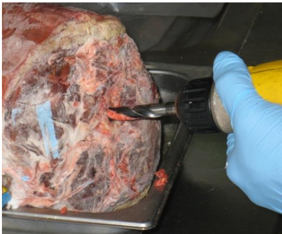
Figure 30 Drilling and insertion of threaded rod into medullar canals during preparation
