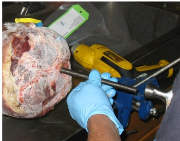
Figure 30 Drilling and insertion of threaded rod into medullar canals during preparation
