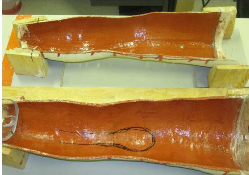
Figure 36 Tape mould cut along medio-lateral plane and prepared for moulding external foam shell on a custom built fixture
