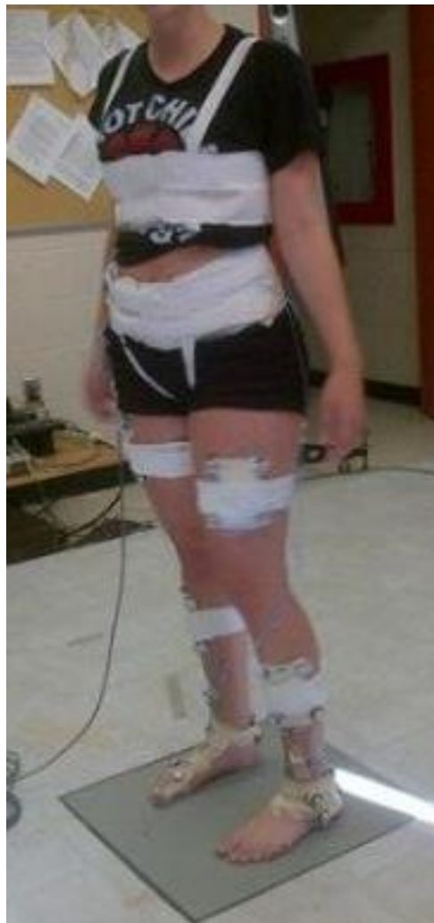
Figure 23 Athlete instrumented with infrared markers during motion capture
