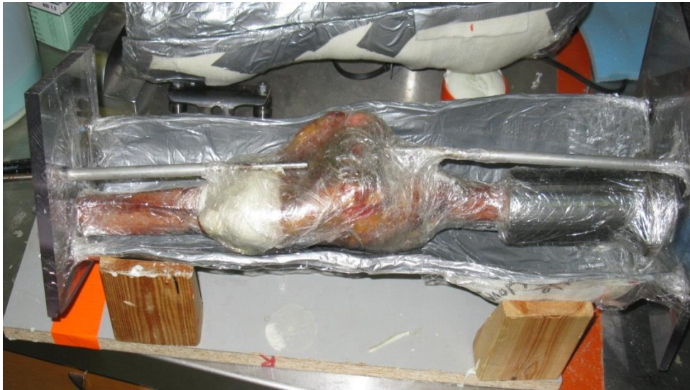
Figure 44 Prepared cadaver specimen oriented and located in tape mould along with aluminum tube conduits for muscle actuator cables
