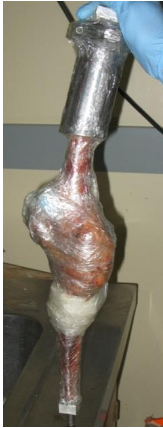
Figure 43 Cadaver knee wrapped with clear tape prior to foam shell moulding
