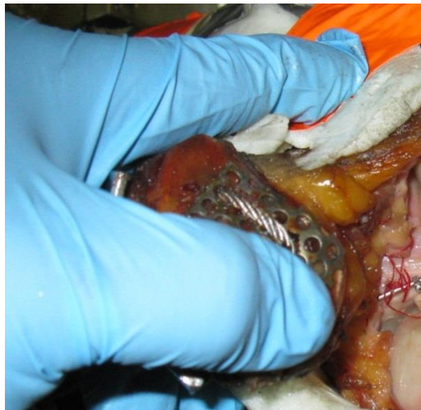
Figure 55 Metal shims layered on both inferior articulation portion and superior portion of patella to avoid stress concentration around holes drilled in patella and muscle actuator cable inserted through the holes drilled in patella
