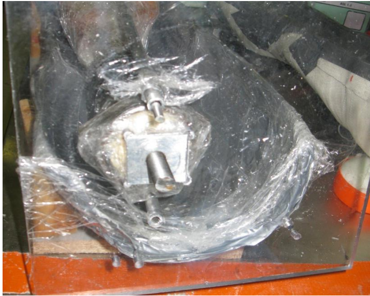
Figure 45 Aluminum tubes located in holes drilled in end plates while cadaver knee specimen and locator blocks remain aligned to tape mould
