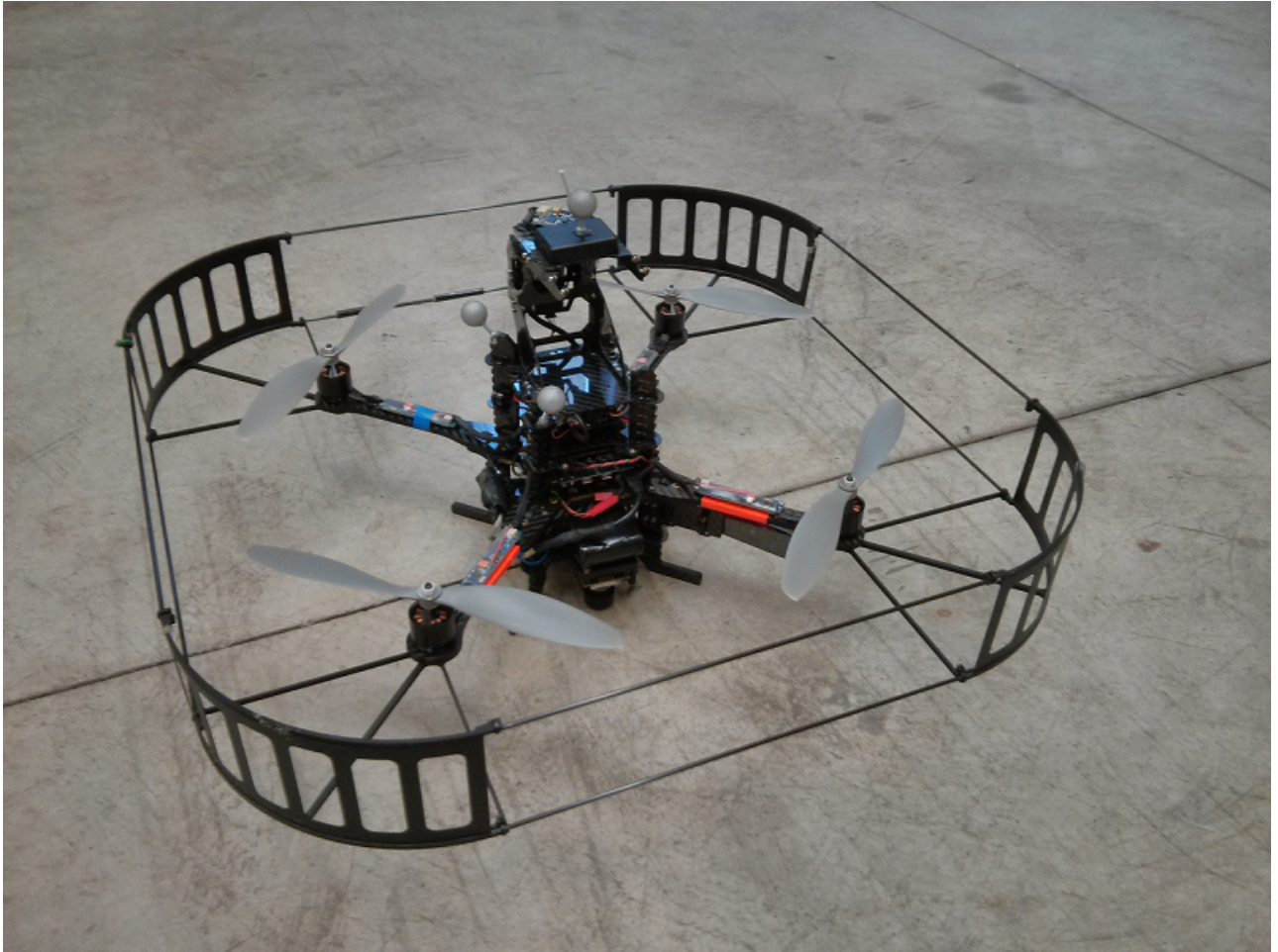
Figure 4.1: Pelican quadrotor used in experiments
