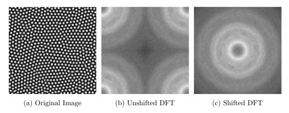
Figure 2.1: Fourier Shift: Shifting the spectral density allows frequencies to be grouped into circles around the image centre. In figure (c), the distance r from the image centre represents frequency, and the brightness reflects the amplitude of the original image at that frequency.
