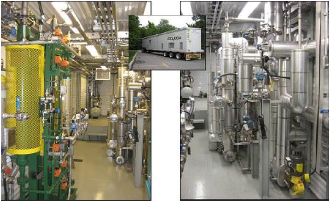
Figure 2-6 Trailer mounted CanCO 2 unit at operation at CanmetENERGY, Ottawa
