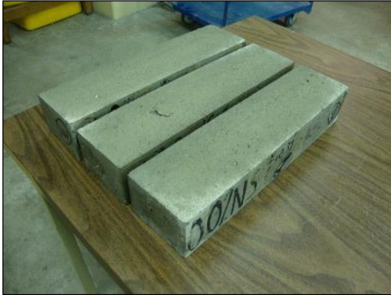
Figure 4-41: Prisms with 0.0% nanosilica after 324 cycles of freezing and thawing w/c = 0.39
