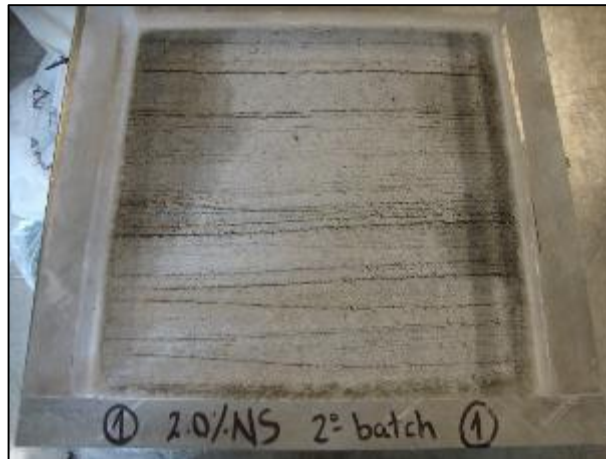
Figure D11: Picture after 25 cycles – 2.0% nanosilica, sample 1, second batch
