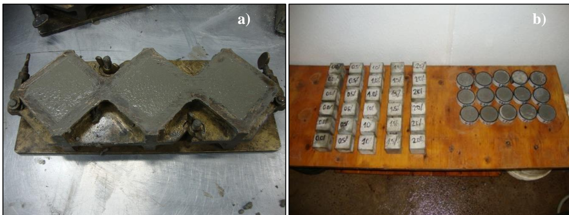
Figure 3-4: a) Casting of cube specimens and b) mortar samples inside the curing room
