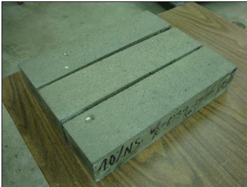
Figure 4-42: Prisms with 1.0% nanosilica after 324 cycles of freezing and thawing w/c = 0.39
