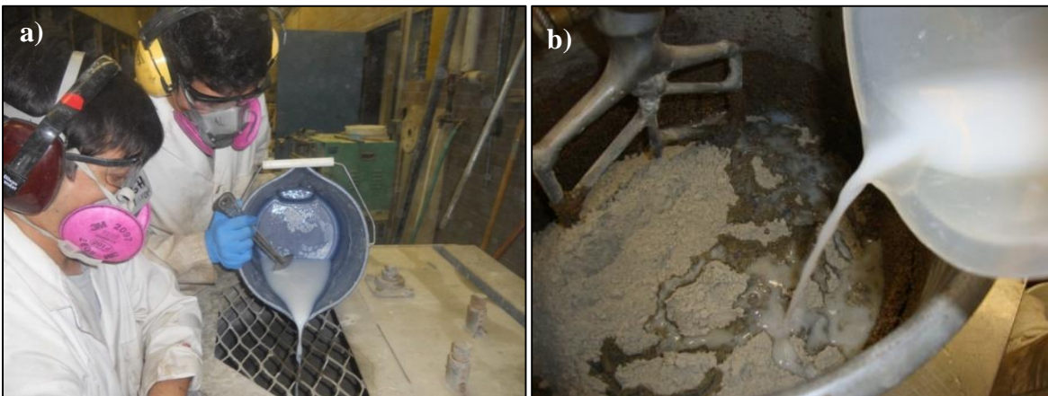
Figure 3-1: Nanosilica incorporates in water during mixing a) in concrete mixes and b) mortars
