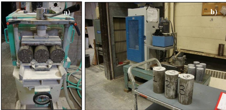
Figure 3-5: a) Grinding the cylinders before compressive strength testing and b) the compressive strength machine
