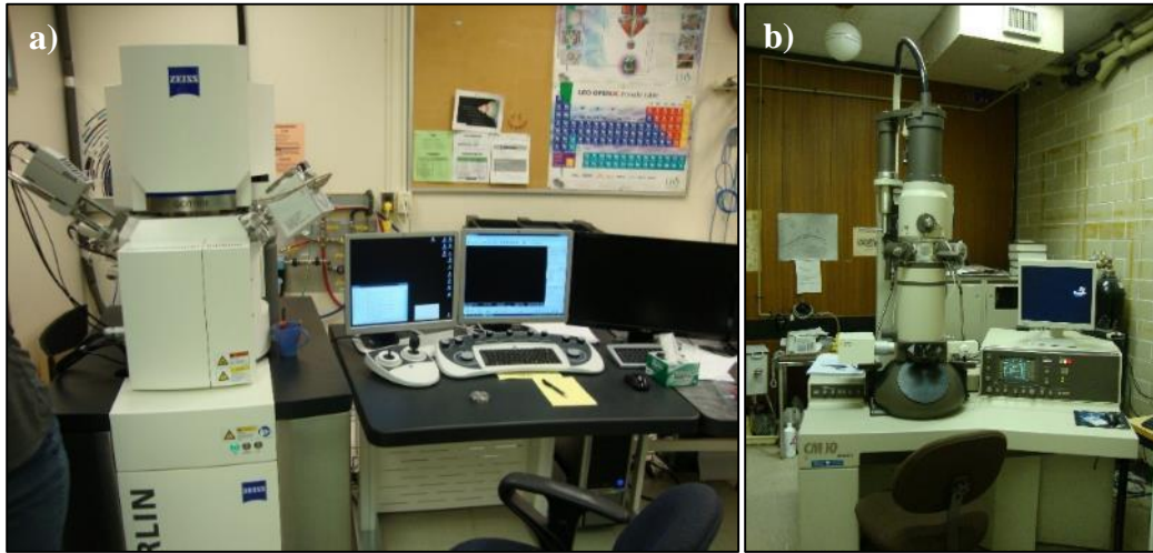
Figure 3-12: Pictures presenting a) Scanning Electron Microscope (SEM) and b) Transmission Electron Microscope (TEM) from UW
