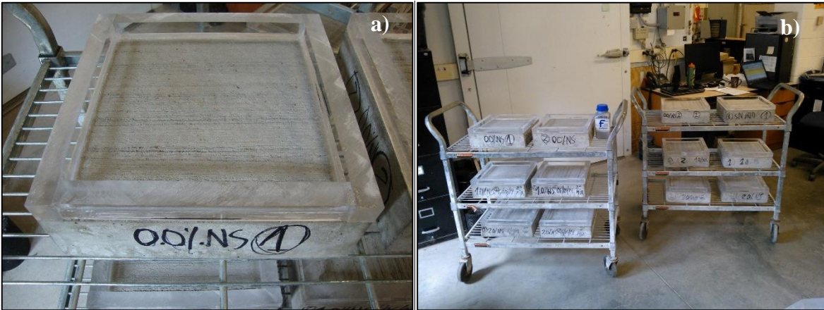
Figure 3-8: a) Sample with the dike of Plexiglass and b) samples before the first cycle began
