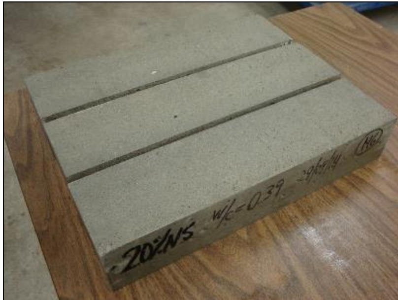
Figure 4-43: Prisms with 2.0% nanosilica after 324 cycles of freezing and thawing w/c = 0.39
