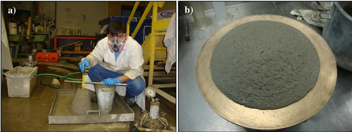
Figure 3-2: a) Slump test in concrete and b) flow consistency in mortars
