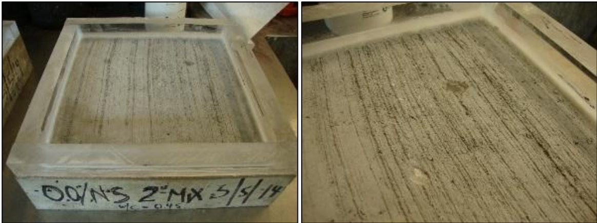
Figure 4-46: Scaling evaluation after 25 cycles, 0.0% nanosilica, sample number 2, second set of samples (second batch)
