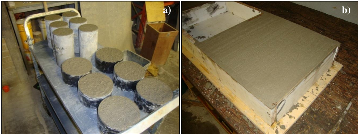
Figure 3-3: a) Casting of samples for compressive strength and noise absorption and b) casting of slabs for scaling resistance
