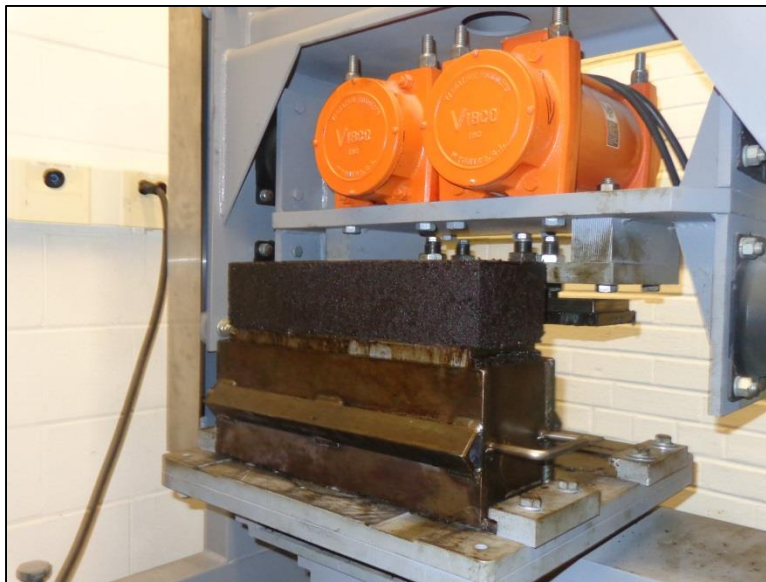
Figure 3-23 Asphalt Vibratory Compacted Beam
