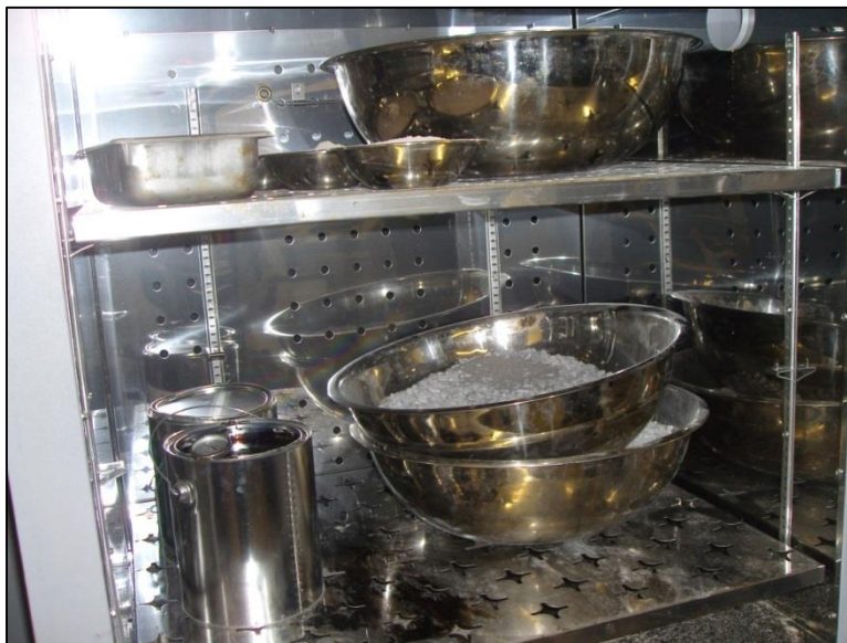
Figure 3-17 Heating Asphalt and Aggregates
