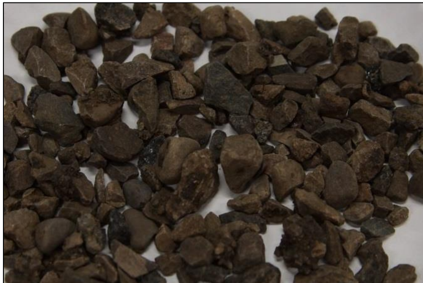
Figure 6-8 RAP Sample after Partial Extraction
