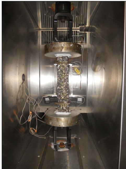
Figure 4-1 CPATT TSRST Frame and Environmental Chamber
