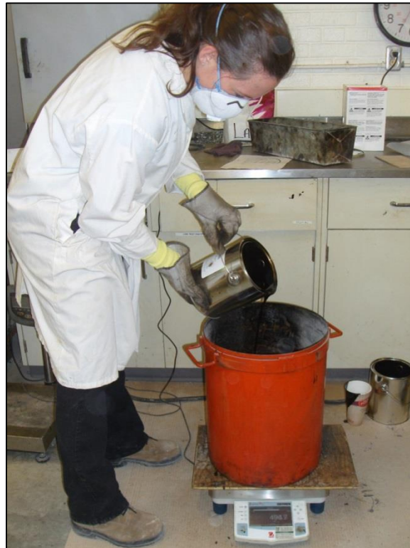
Figure 3-19 Adding Hot Asphalt Binder
