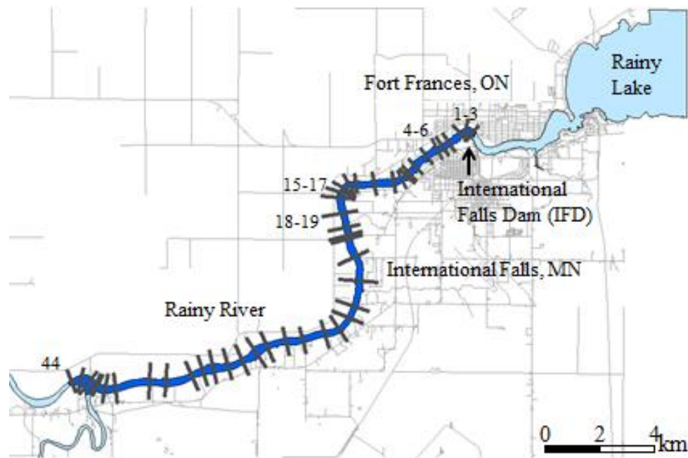
Figure 5.1 The Rainy River is located at the border of Fort Frances, ON, and International Falls, MN. The International Falls dam and the confluence with Little Fork River represent the boundaries of the study reach. Grey bars indicate locations where hydraulic cross-sections (1 to 44). Cross-sections 1-3 and 4-6 denote lake sturgeon spawning locations. Cross-sections 1-3, 15-17 and 18-19 denote walleye spawning locations.
