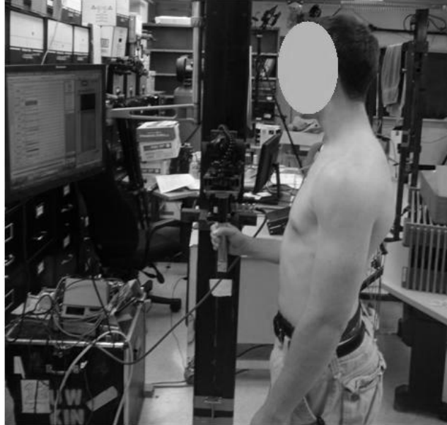
Figure 34 A participant grasps the handle attached to the tri-axial force cube and exerts a rotational force - meeting a target displayed by visual force feedback on the computer monitor
