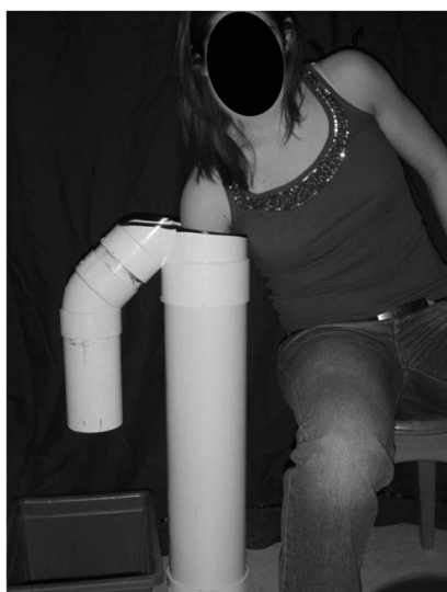
Figure 15 Arm volumeter used to measure arm volume via water displacement. Instrument designed by Lette (2006).
