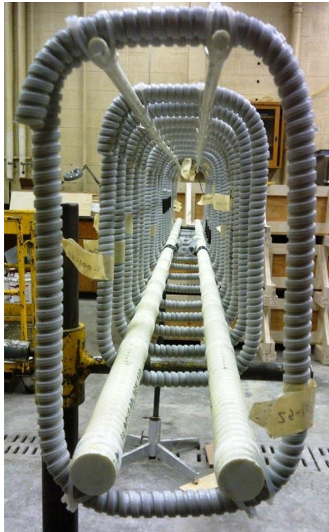
Figure E.181: BM25-150 Rebar Cage Cross-Section Photo
