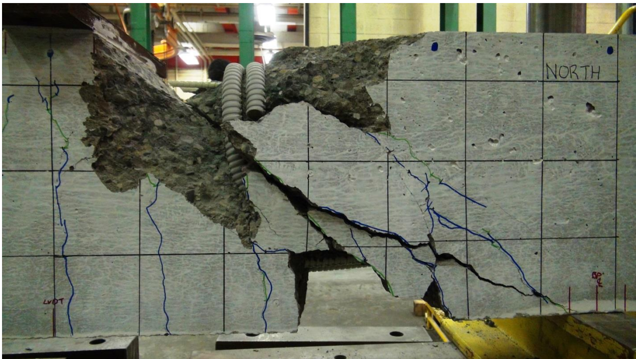
Figure E.225: BM16-s230 Close-up Photo Failure with Spalled Concrete Removed with Stirrup 8 Exposed
