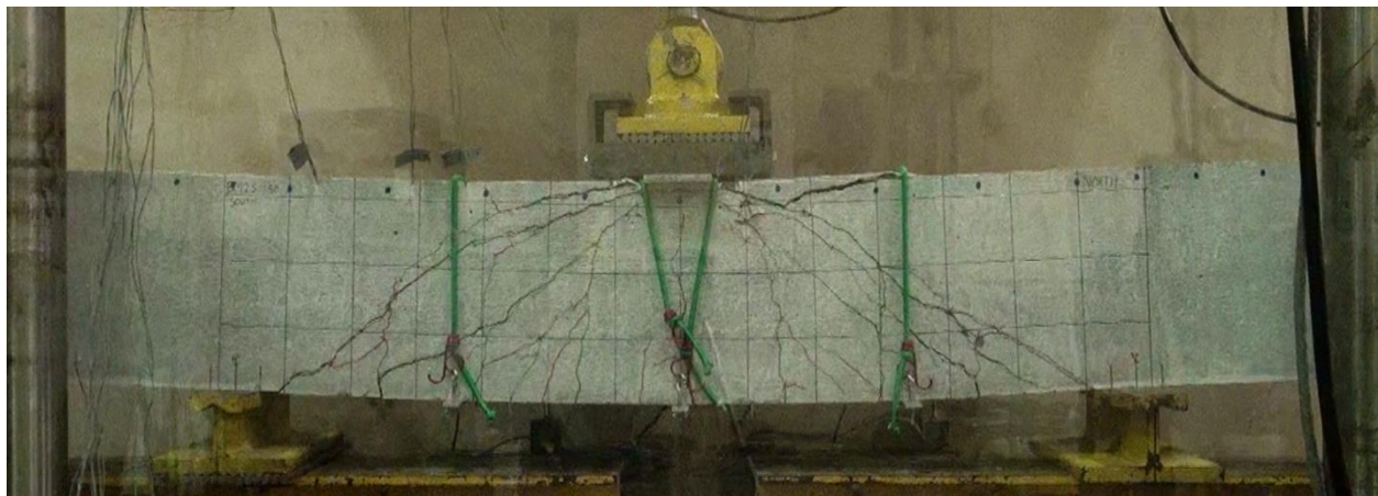
Figure E.164: BM25-150 At Peak Load
