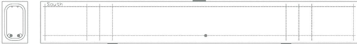
Figure E.41: BM25-INF Schematic of Mid-Span Strain Gauge Locations
