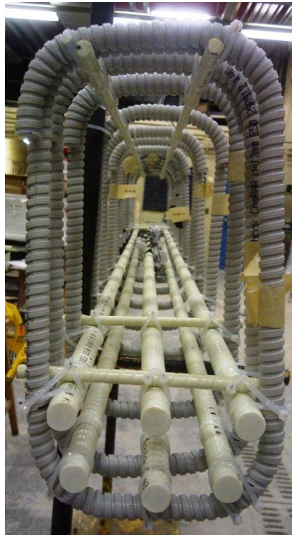
Figure E.159: BM16-150 Rebar Cage Cross-Section Photo
