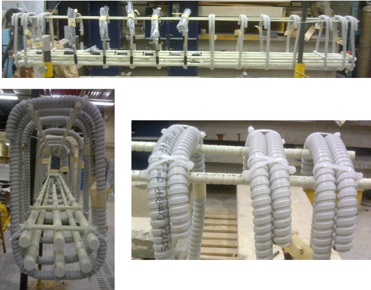
Figure 3.4: Collection Rebar Cage Photos for Beam BM16-150
