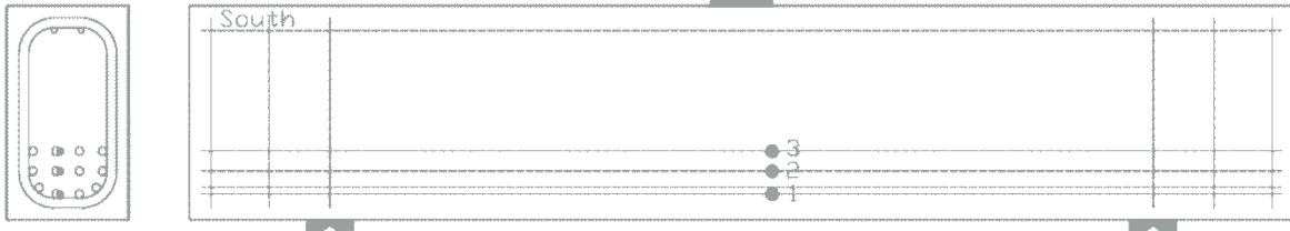
Figure E.9: BM12-INF Schematic of Mid-Span Strain Gauge Locations
