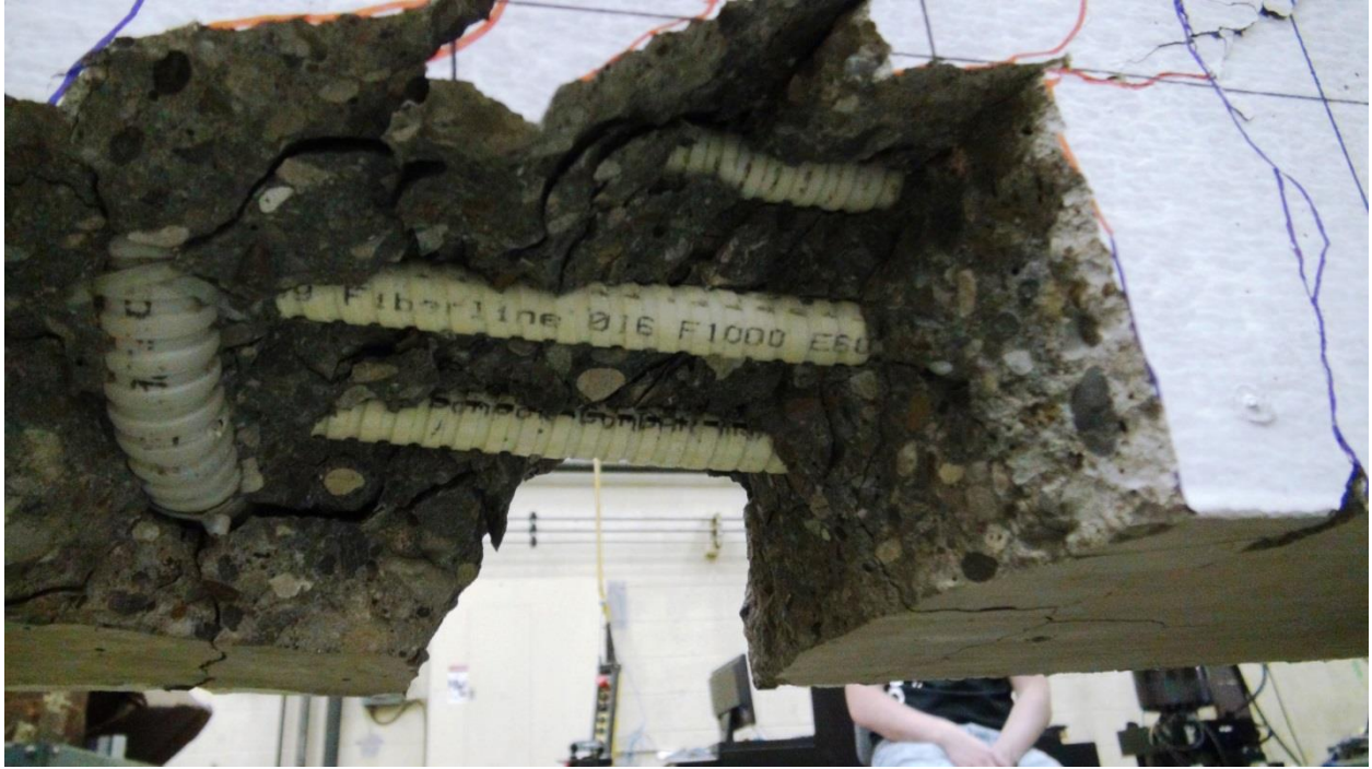
Figure E.226: BM16-s230 Photo of Exposed Stirrup 9 and Longitudinal Bars
