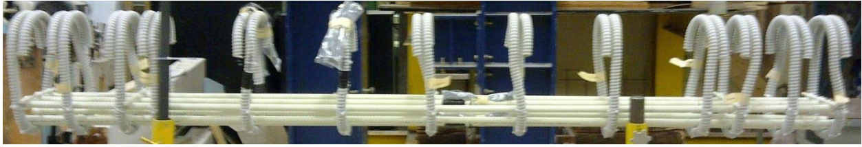
Figure E.222: BM16-s230 Rebar Cage Elevation Photo Top framing bar not pictured.
