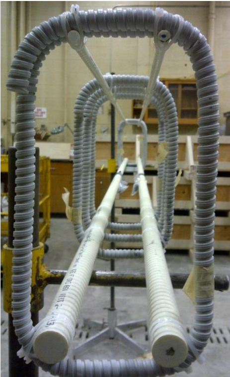
Figure E.45: BM25-INF Rebar Cage Cross-Section Photo
