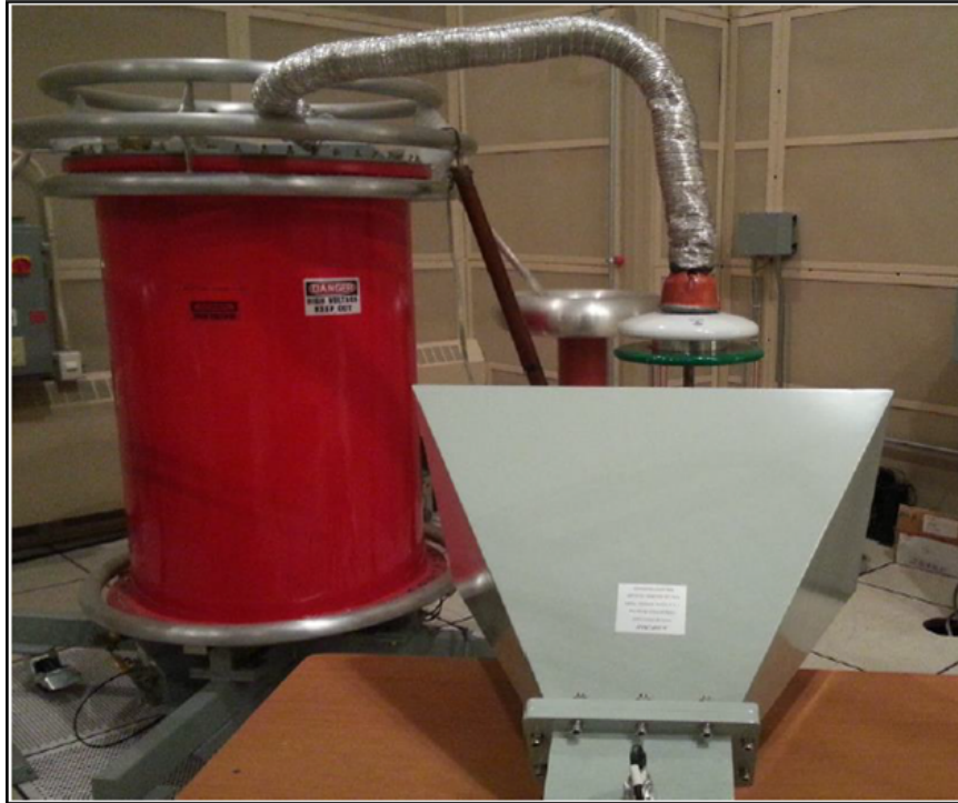
Figure 3.13: Test Setup showing the antenna, test transformer and the insulator sample under test.
