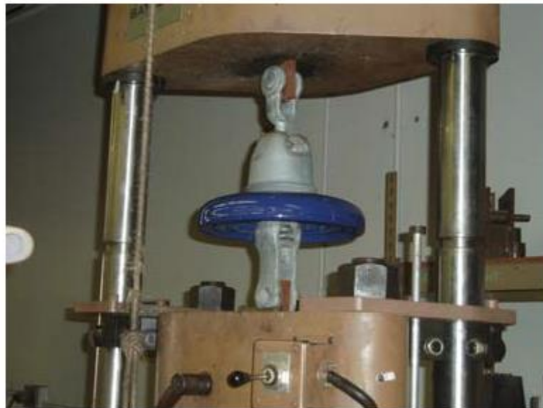
Figure 1.8: Tensile Test setup[14]
