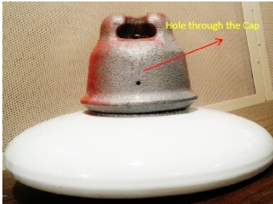
Figure 3.5: Insulator with a hole through the cap.
