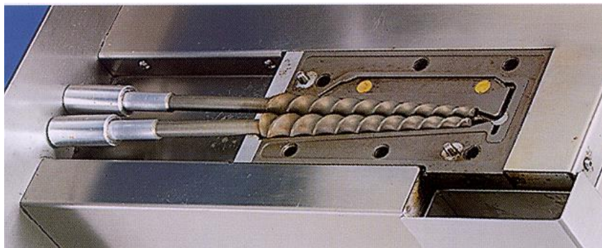
Figure 3.3 The view inside Haake Minilab extruder (Thermo Electron Corporation)
