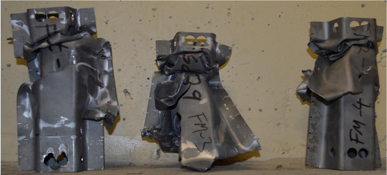
Figure 57. Final deformed shapes of the three crushed fully cooled specimens
