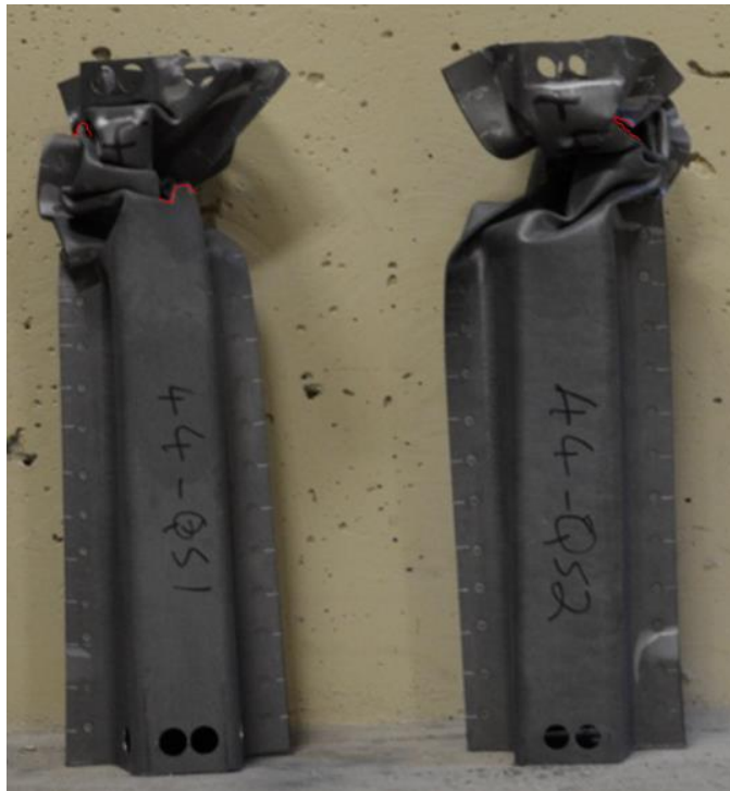
Figure 73. Final deformed shapes of the two crushed single soft zone 400°C specimens. Locations of cracking are outlined in red
