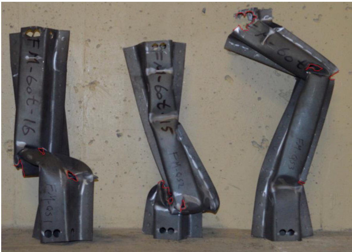
Figure 70. Final deformed shapes of the three crushed fully cooled specimens. Locations of cracking are outlined in red
