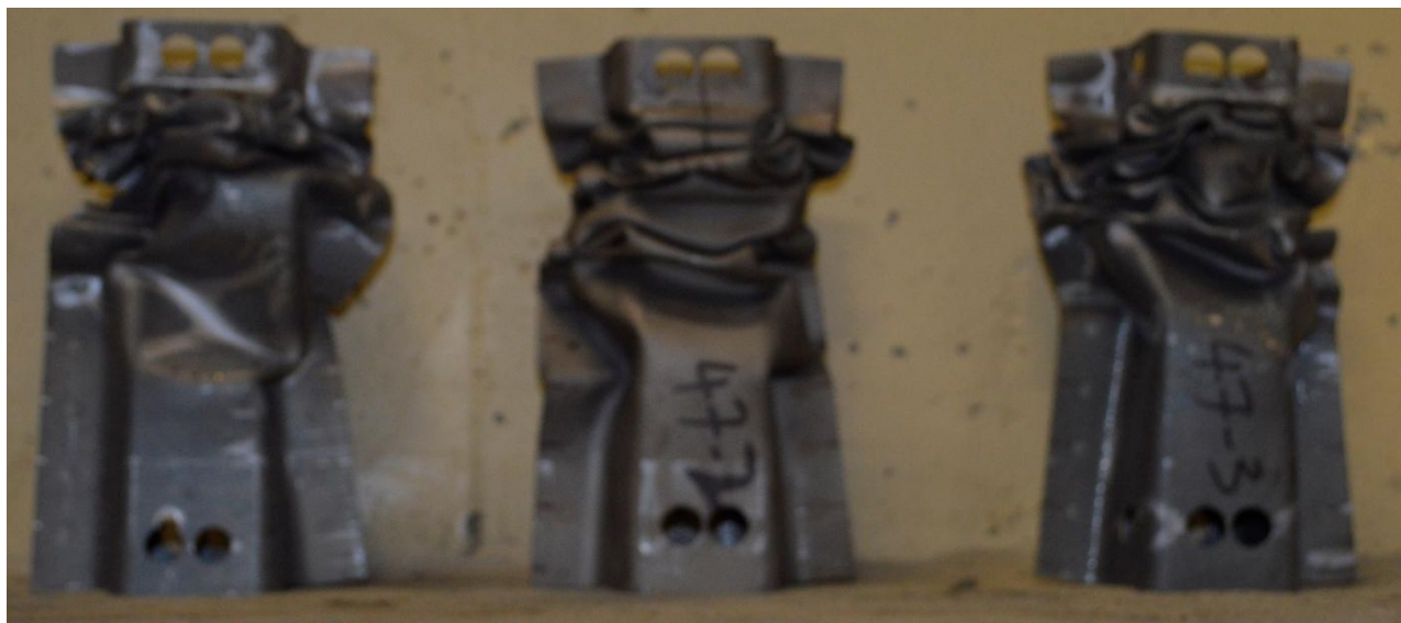
Figure 66. Final deformed shapes of the three crushed graded soft zone specimens
