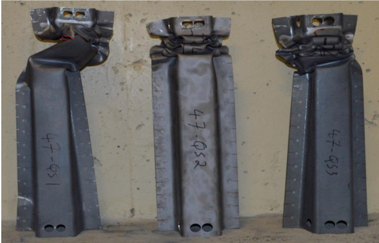
Figure 79. Final deformed shapes of the three crushed graded soft zone specimens. Locations of cracking are outlined in red.
