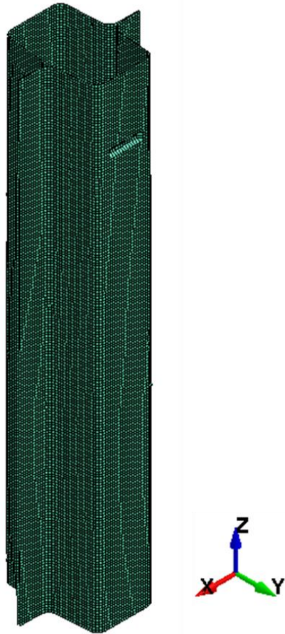
Figure 38. Final mesh in the axial crush specimen
