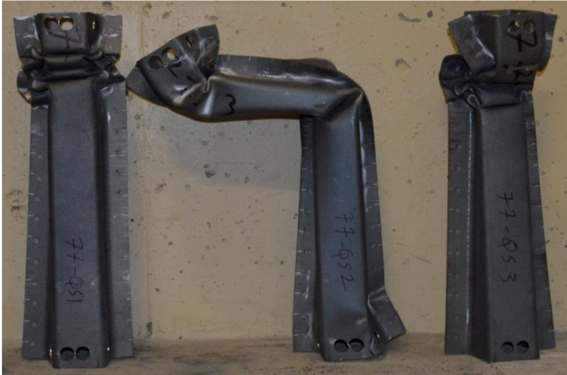
Figure 76. Final deformed shapes of the three crushed single soft zone 700°C specimens
