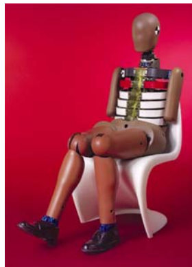
Figure 2.17 WorldSID surrogate dummy
