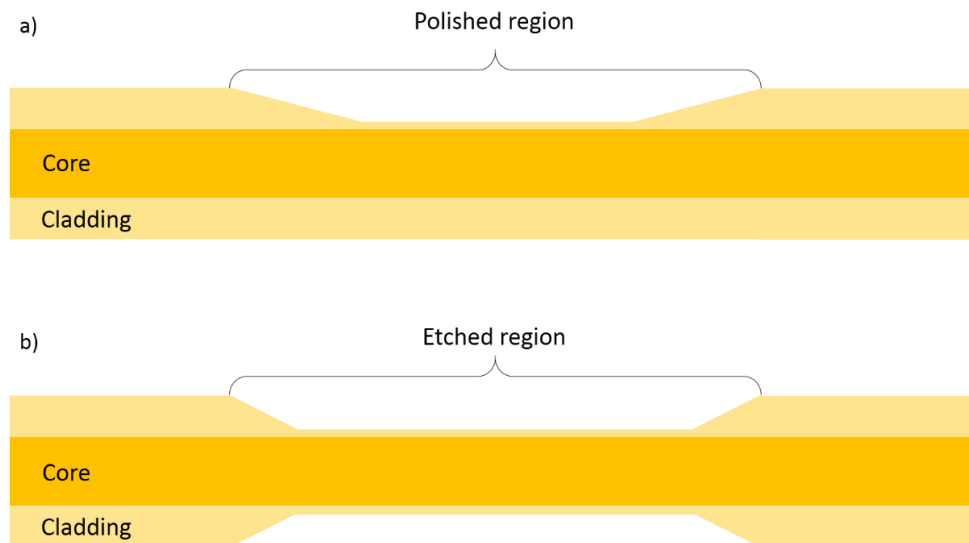
Figure 3: Illustration of side-polished fiber (a) and etched fiber (b) showing the sensing region as either polished or etched.
