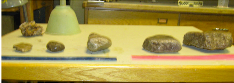
Figure 46: Gravel particles used in VII bottom depth measurements
