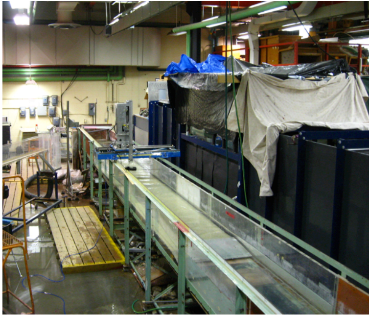
Figure 32: Laboratory flume used for experiments
