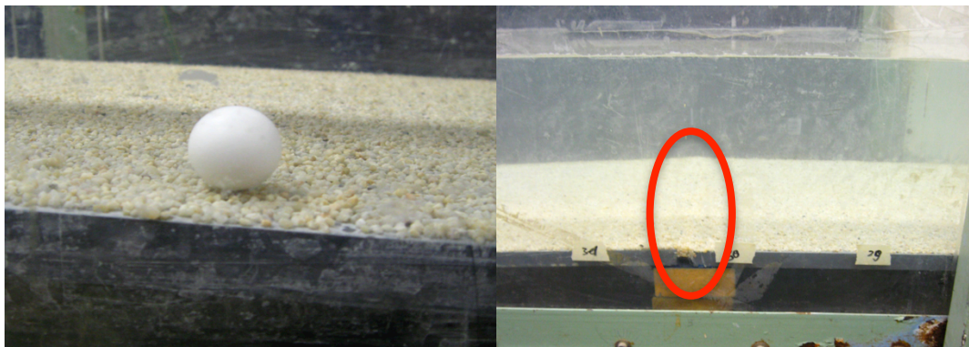
Figure 34: Spherical particle and sand grains on PVC sheets (left) and loose sand covering transition between sheets (right)
