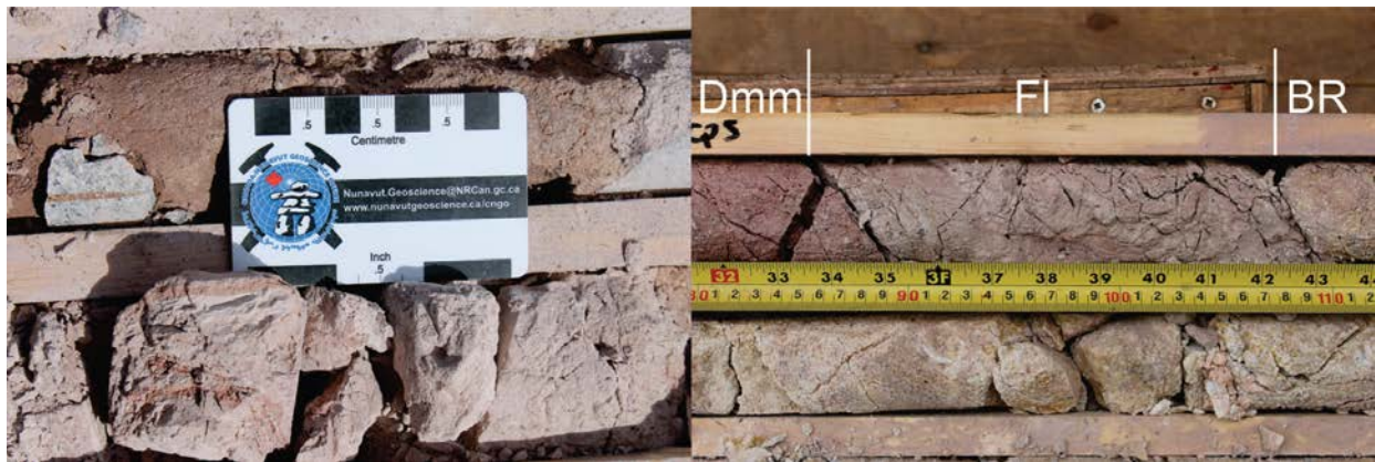
Figure 3-11: Examples of the laminated fine-grained sediments encountered in drillholes ABR-012 (left) and AYA-009 (right) at Ayra. Note contacts are angled within the drillcore due the inclined path of drilling.
