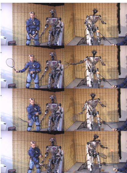
Figure 3.14: Left column: Teacher demonstration of a tennis swing. Right column: Imitation of a tennis swing by a humanoid robot, taken from [159].
