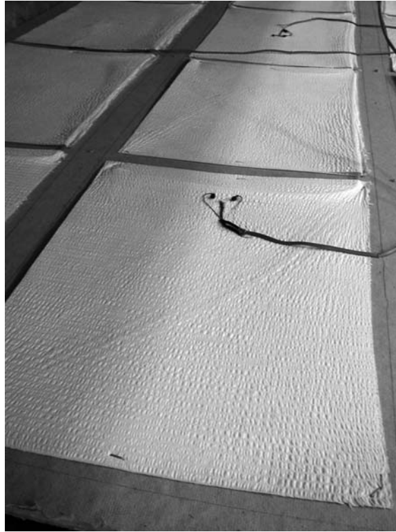
Figure A-4: Wetting Paper after 4 Tests
