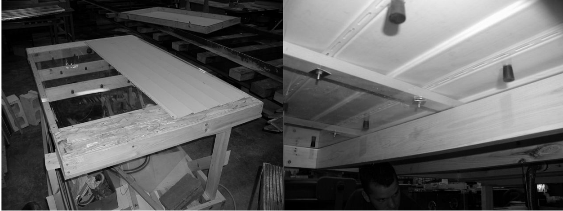
Figure 6-4: Test Rig During Setup for In-Plane Horizontal Flow (left - view from top, right - view from bottom)
