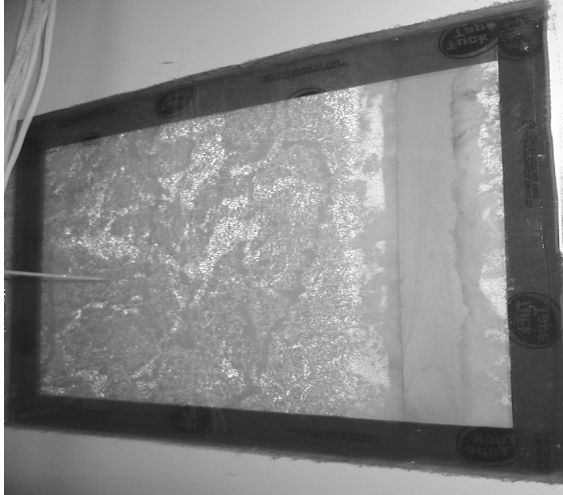
Figure 8-19: Condensation Observed on View Window
