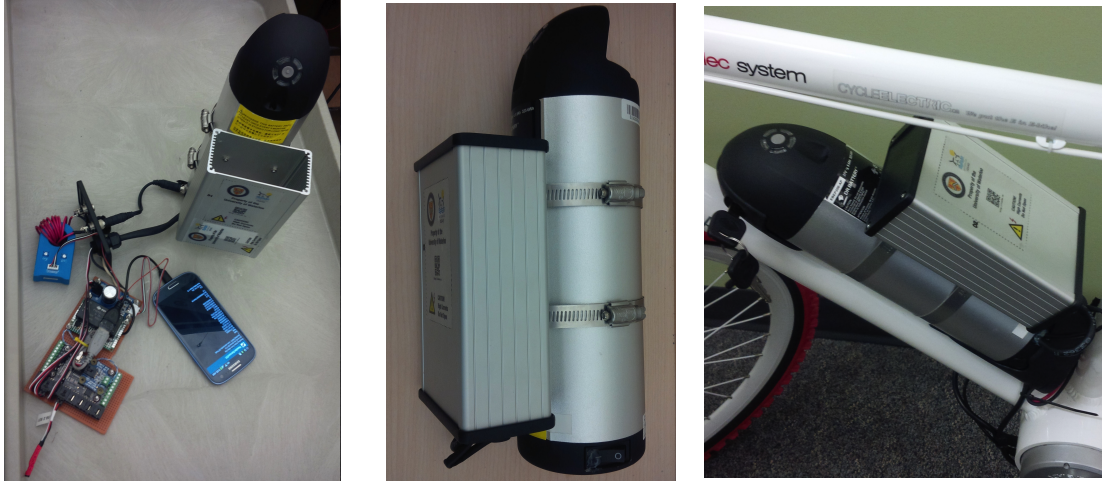
Figure 8.3: eBike sensor kit assembly. Left: connected sensors, middle: sensors enclosed in weather proof case, right: battery + sensors + case assembly shown on bike.
