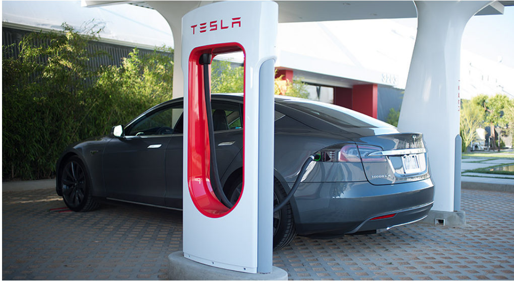
Figure 2.1: A Tesla Model S charging at a Level 3 PEVSE pillar ("Supercharger"). Image source: Tesla [Tes14c].
