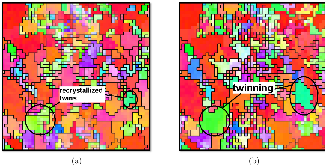
Figure 7.9: Crops from the final full EBSD samples after simulations with different mobility functions (a) step function (b) one peak function
