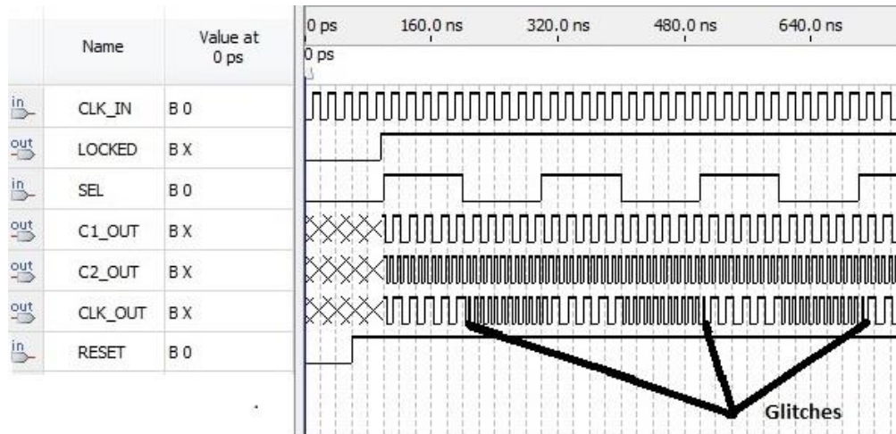
Figure 3.6 Waveform simulation showing presence of glitch during clock switching
