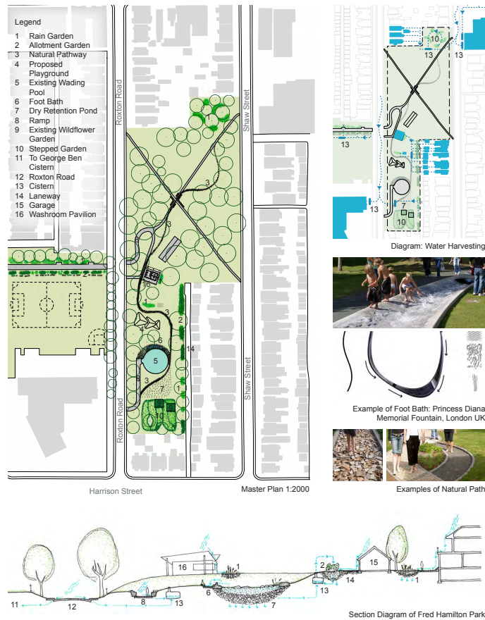
FIG. 95 "The Water Harvest," a masterplan for incremental water harvesting systems for Roxton Road Parks in Toronto. Drawing by F_RMIlab.
