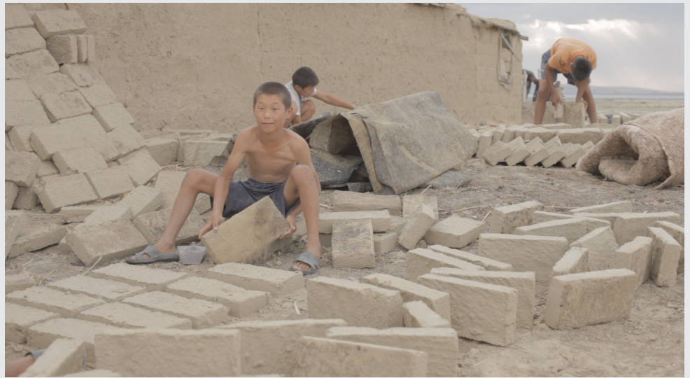
FIG. 75 Mud bricks made from loess, an aeolian clay found in the Aral region.
