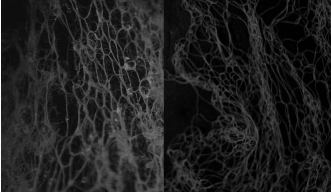
FIG. 100 Tests showing knitted prototypes in wool/mohair (right) and nylon (left) fibres. Wool droplets collect and bead while the nylon net simply becomes saturated.
