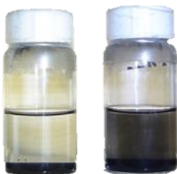
Figure 6.17 Colloidal stability in methanol of Inco 85109 Ni nanopowder stabilized by (left) PEO 6.6k - b -PS 700 - b -PEO 6.6k after 4 h, and (right) P2VP 8k - b -PS 6k - b -P2VP 8k after 25 days.
