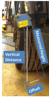
Figure 5.6. Difference between measured height with the height sensor and vertical distance between sensor and ground
